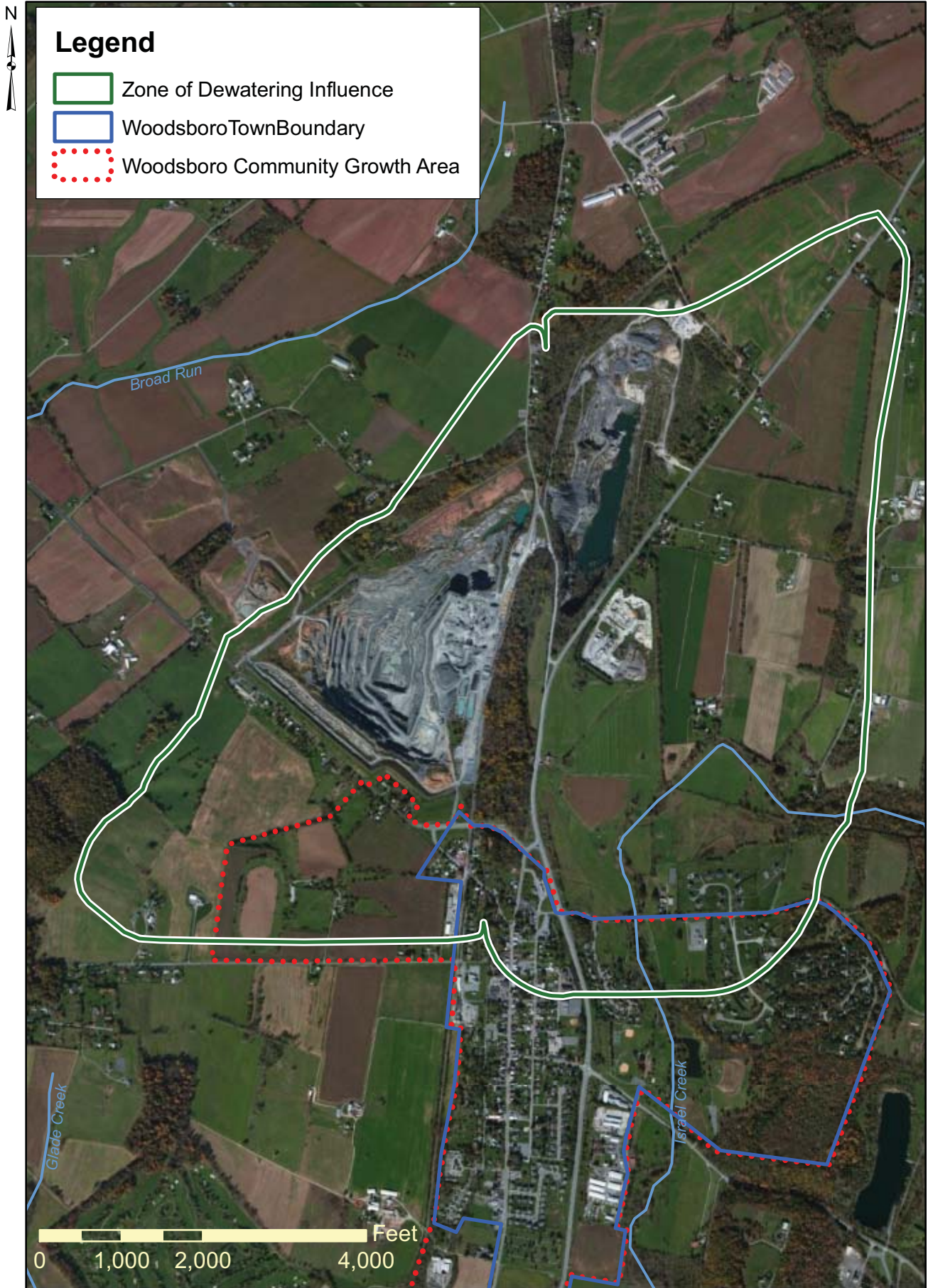
Figure 5 Quarries and Zone of Dewatering Influence, Woodsboro, MD
