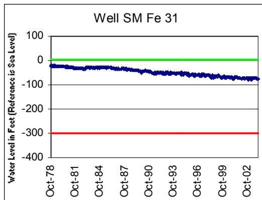
Figure E-6. Hydrograph Records of USGS/MGS Monitoring Wells in the Aquia Formation Showing Current Water Levels, Pre-pumping conditions and the 80% Management Level.
