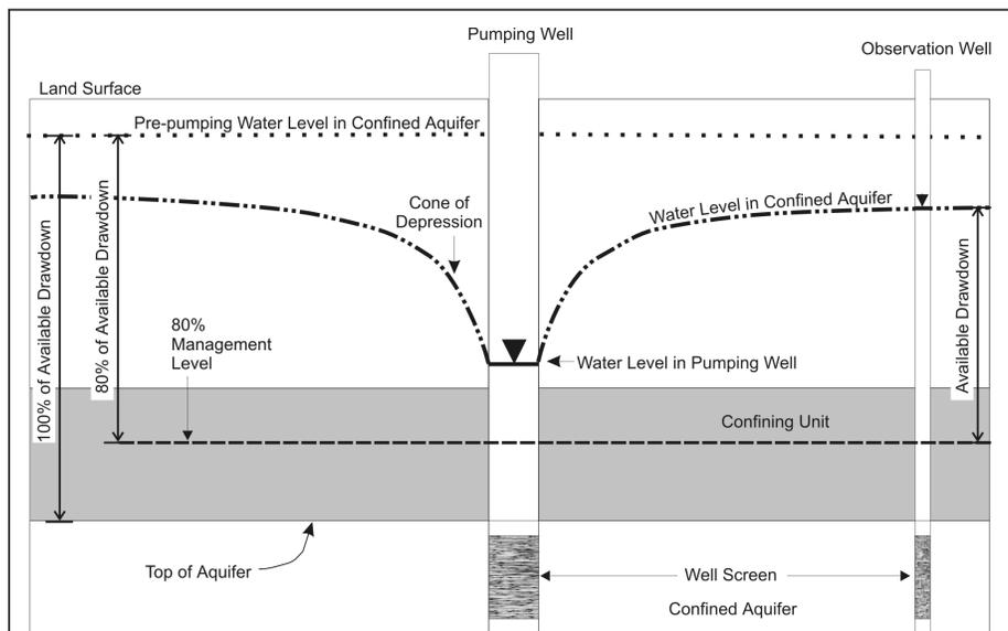
Figure E-4. Schematic Illustration of the 80% Management Level in the Confined Aquifers. The water level rises above the top of the aquifer because it is under pressure and is lowered due to withdrawals from the pumping well. The water level measured at the pumping well is much lower than the water level in the observation well due to the formation of a cone of depression.
