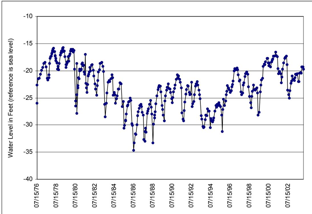
Figure E-11. Hydrograph showing water level decline and recovery in Monitoring Well SM Df 66 in the Piney Point aquifer (see Figure E-5 for well location.)
