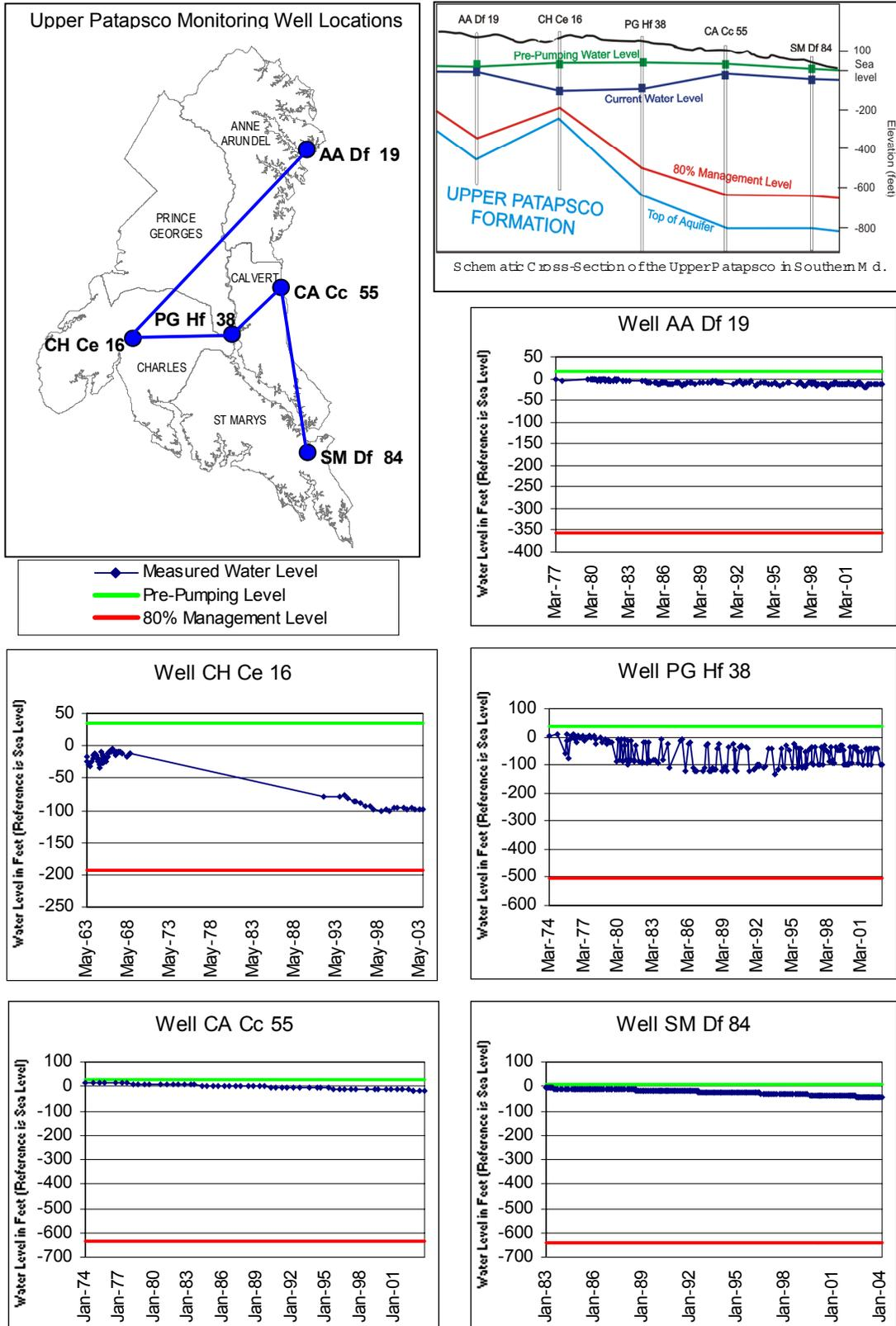
Figure E-8. Hydrograph Records of USGS/MGS Monitoring Wells in the Upper Patapsco Formation Showing Current Water Levels, Pre-pumping conditions and the 80% Management Level.
