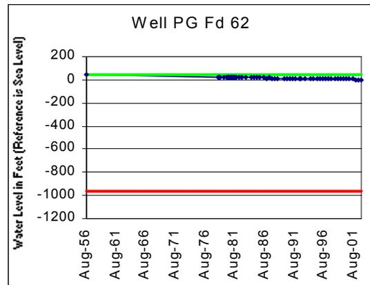
Figure E-10. Hydrograph Records of USGS/MGS Monitoring Wells in the Patuxent Formation Showing Current Water Levels, Pre-pumping conditions and the 80% Management Level.
