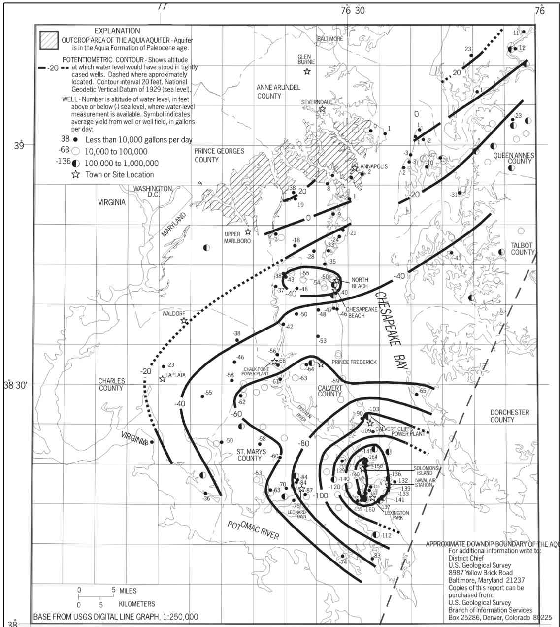
Figure E-12. Potentiometric Surface Map of the Aquia Aquifer (Curtin et al. 2002)
