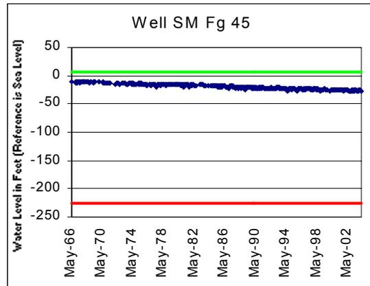
Figure E-5. Hydrograph Records of USGS/MGS Monitoring Wells in the Piney Point Formation Showing Current Water Levels, Pre-pumping conditions and the 80% Management Level.
