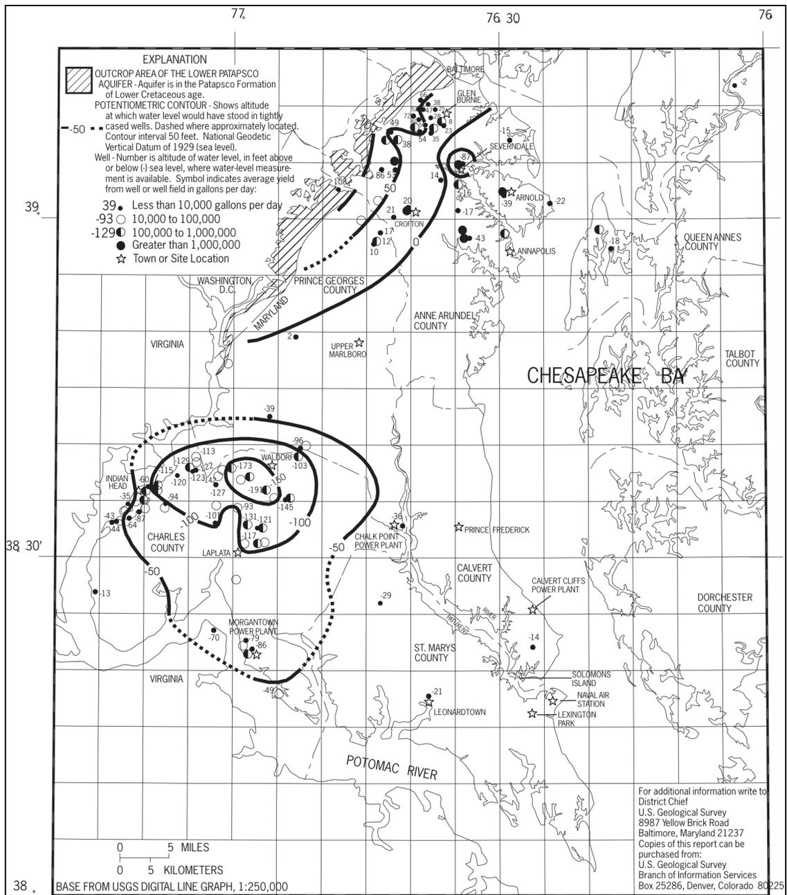
Figure E-13. Potentiometric Surface Map of the Lower Patapsco Aquifer (Curtin et al. 2002)
