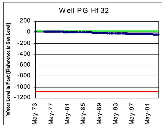
Figure E-9. Hydrograph Records of USGS/MGS Monitoring Wells in the Lower Patapsco Formation Showing Current Water Levels, Pre-pumping conditions and the 80% Management Level.
