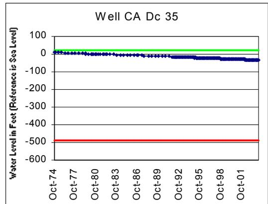
Figure E-7. Hydrograph Records of USGS/MGS Monitoring Wells in the Magothy Formation Showing Current Water Levels, Pre-pumping conditions and the 80% Management Level.
