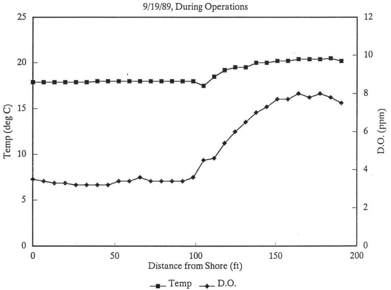
Figure 3-48. Cross-sectional profile for water temperature and dissolved oxygen (D.O.) concentrations 1000 feet below Deep Creek Project tailrace, September 19, 1989.
