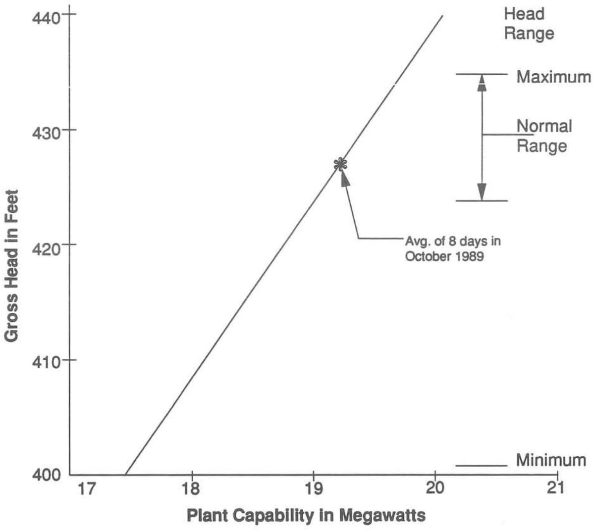
**NOTE:** Outside of the normal head range, the plant capability is uncertain. The depicted curve was derived from known capability at a head of approximately 436 feet and extended in accordance with Figure 9 – "Typical Francis turbine performance – constant speed and full gate," Monograph No. 20, Bureau of Reclamation.
