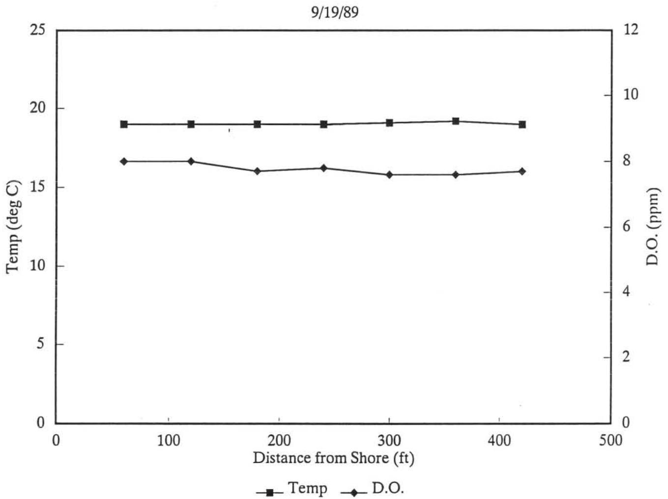
Figure 3-50. Cross-sectional profile for water temperature and dissolved oxygen (D.O.) concentrations at Sang Run, September 19, 1989.
