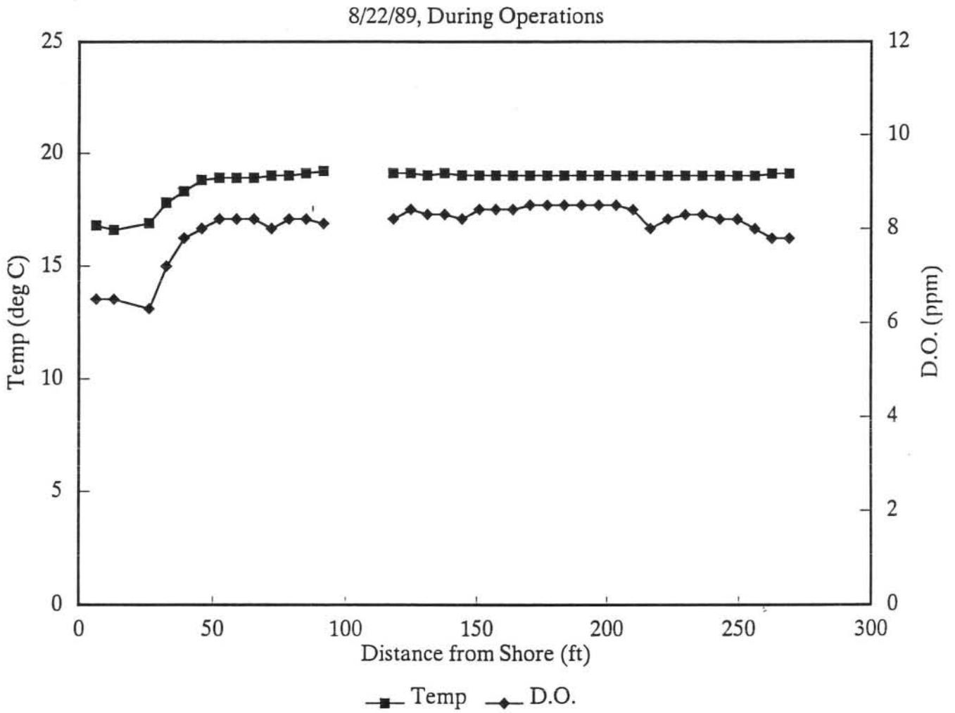
Figure 3-47. Cross-sectional profile for water temperature and dissolved oxygen (D.O.) concentrations 480 feet below Deep Creek Project tailrace, August 22, 1989.
