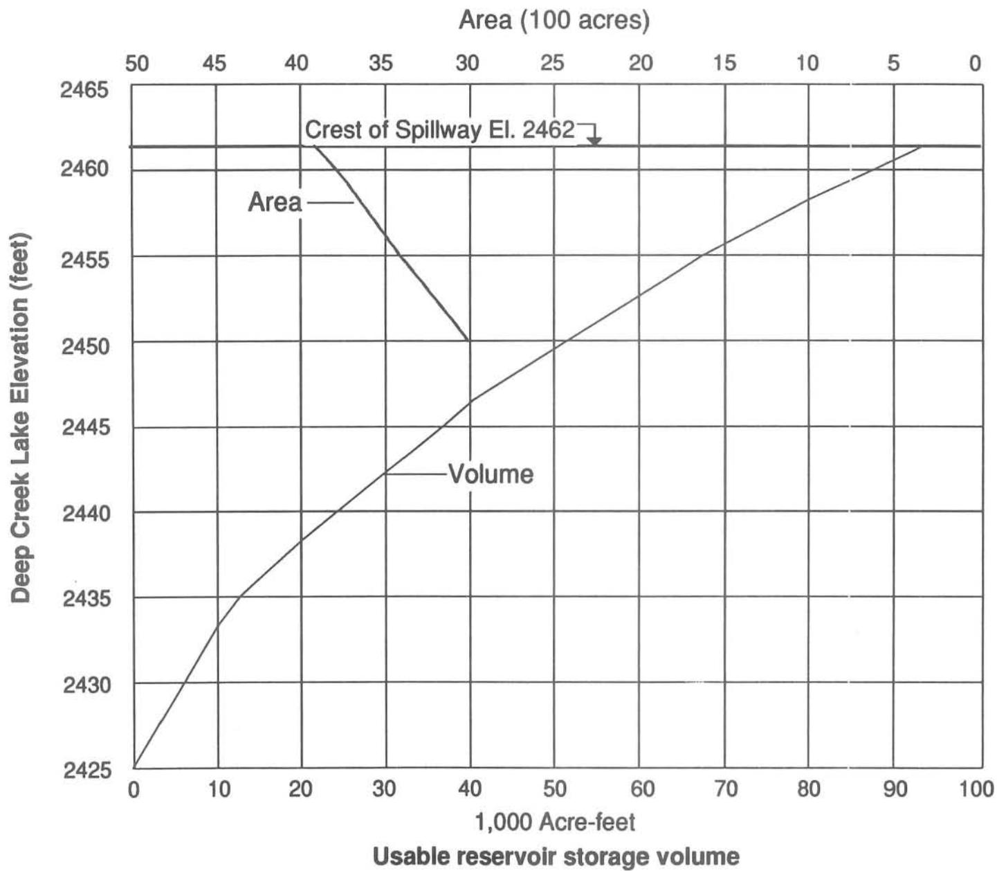
Figure 2-8. Area - capacity - elevation curve.
