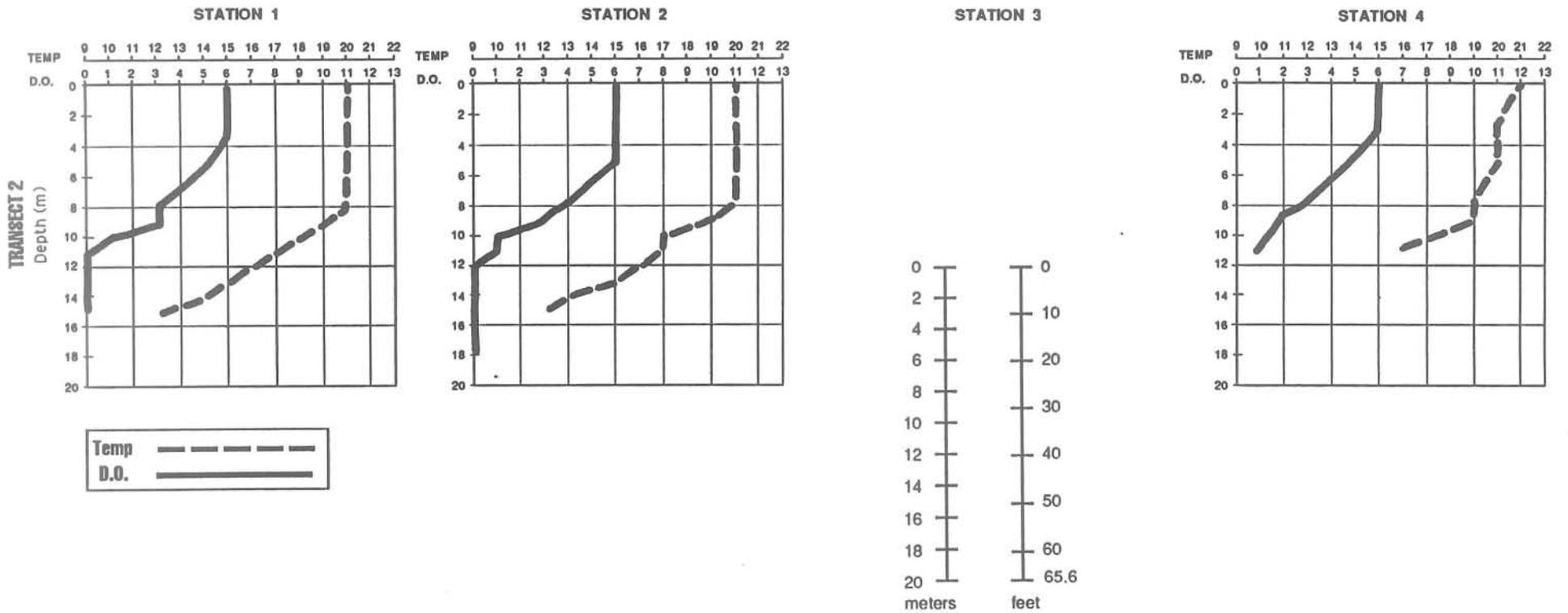
Figure 3-20. Temperature (°C) and dissolved oxygen (ppm) measurements for August 30, 1989, during operation.
