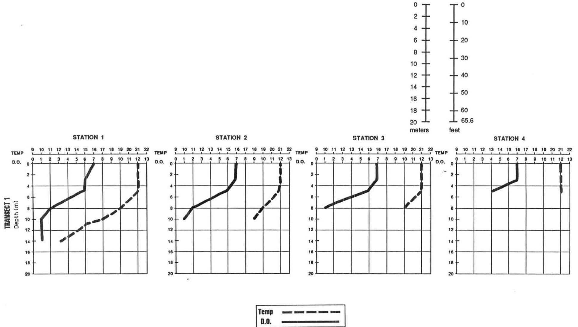
Figure 3-19. Temperature (°C) and dissolved oxygen (ppm) measurements for August 23, 1989, before operation.
