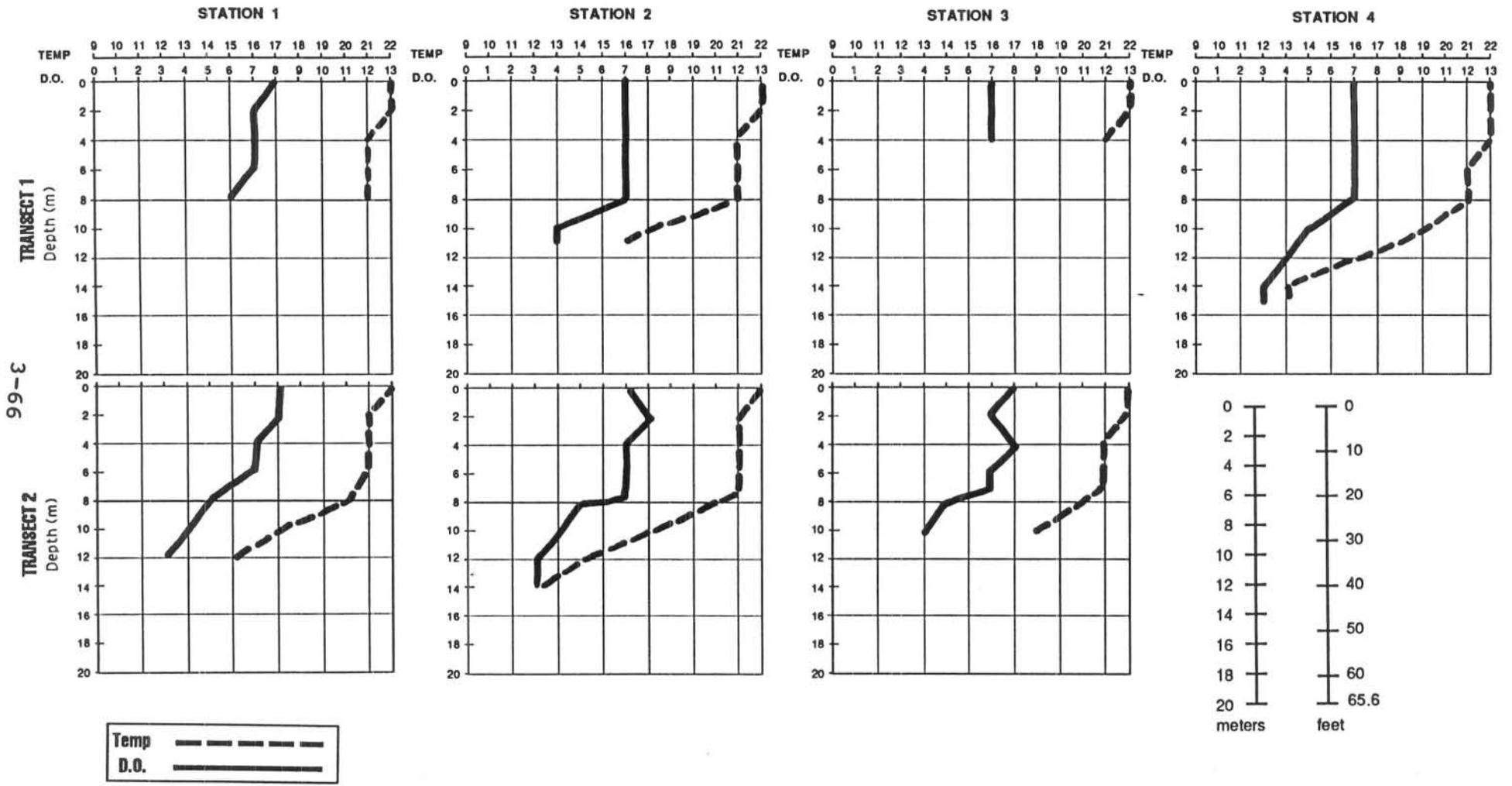
Figure 3-17. Temperature (°C) and dissolved oxygen (ppm) measurements for August 9, 1989, during operation.
