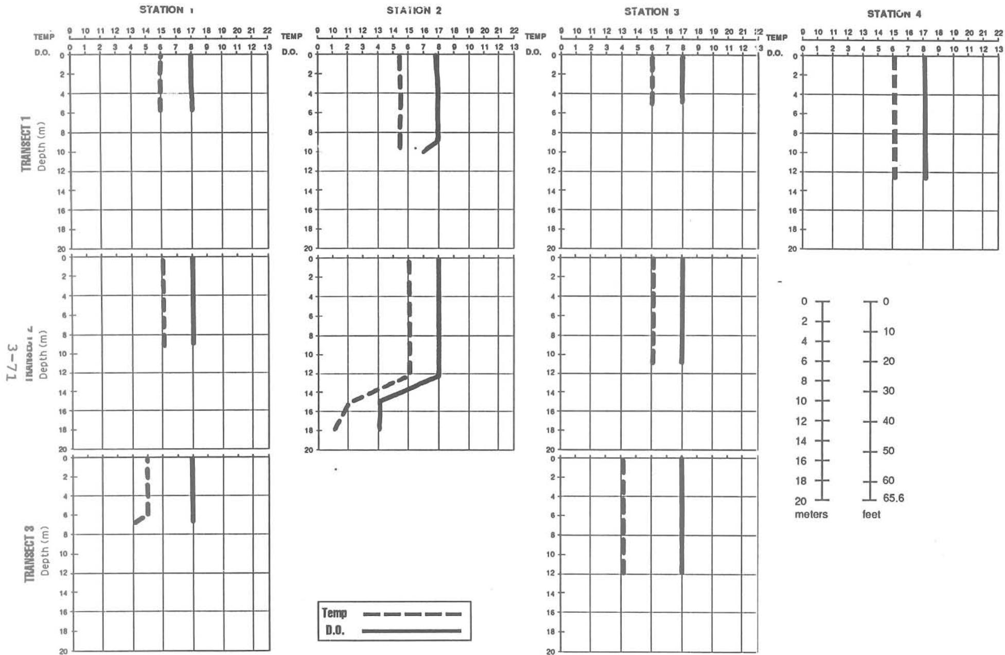
Figure 3-22. Temperature (°C) and dissolved oxygen (ppm) measurements for October 9, 1989, during operation.
