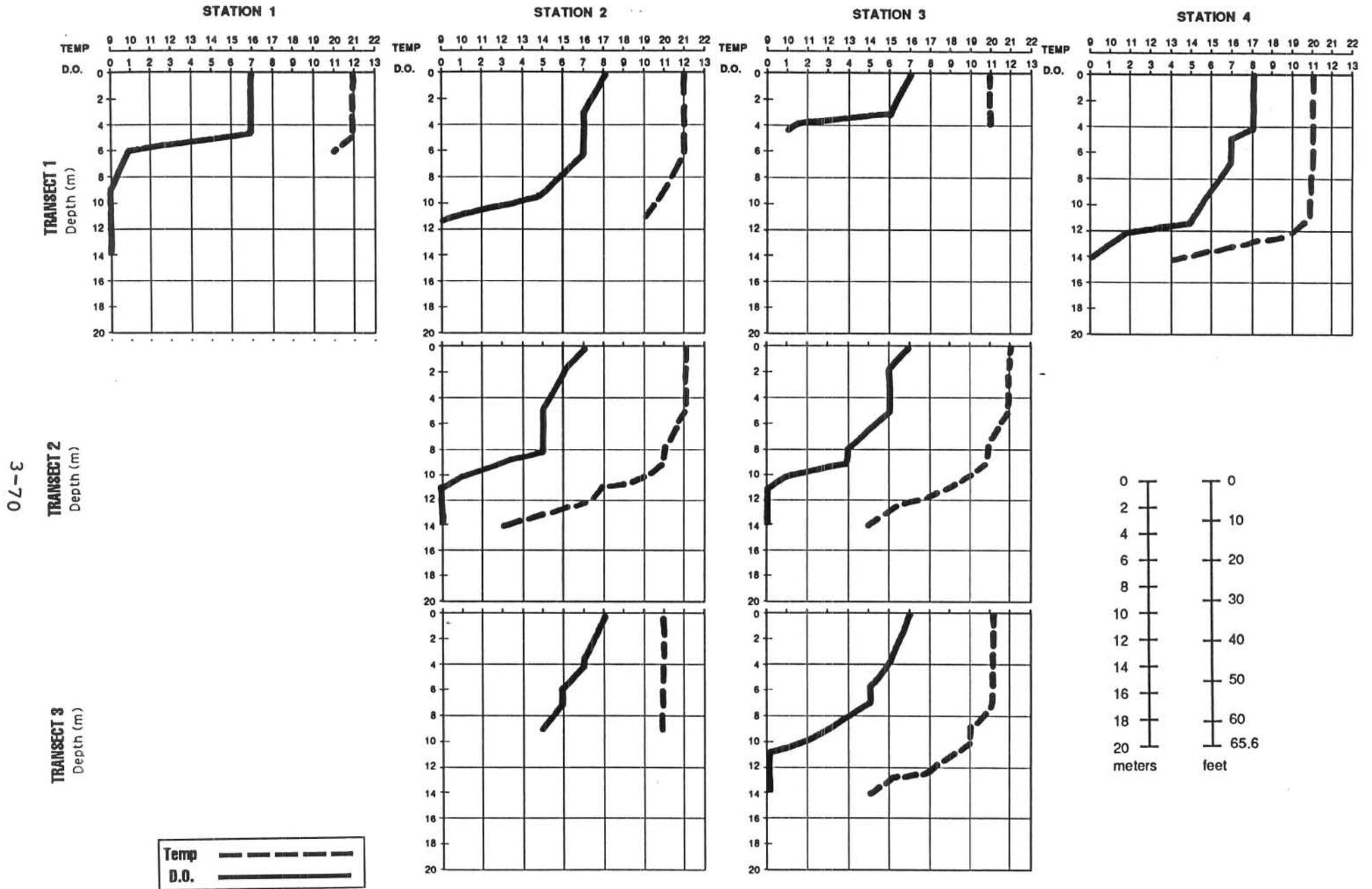
Figure 3-21. Temperature ( $^{\circ}\text{C}$ ) and dissolved oxygen (ppm) measurements for September 18, 1989, during operation.
