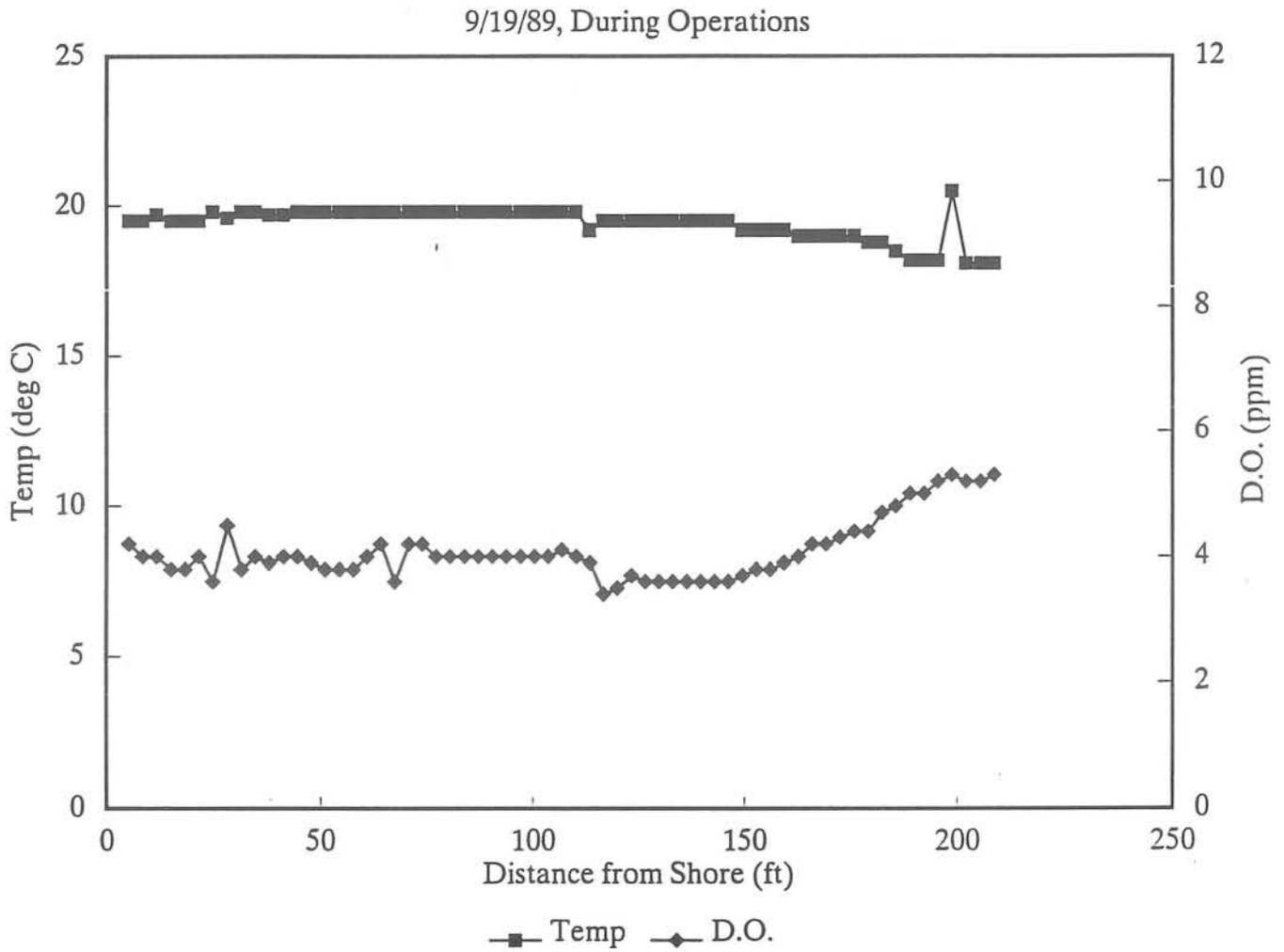
Figure 3-49. Cross-sectional profile for water temperature and dissolved oxygen (D.O.) concentrations 2125 feet below Deep Creek Project tailrace, September 19, 1989.
