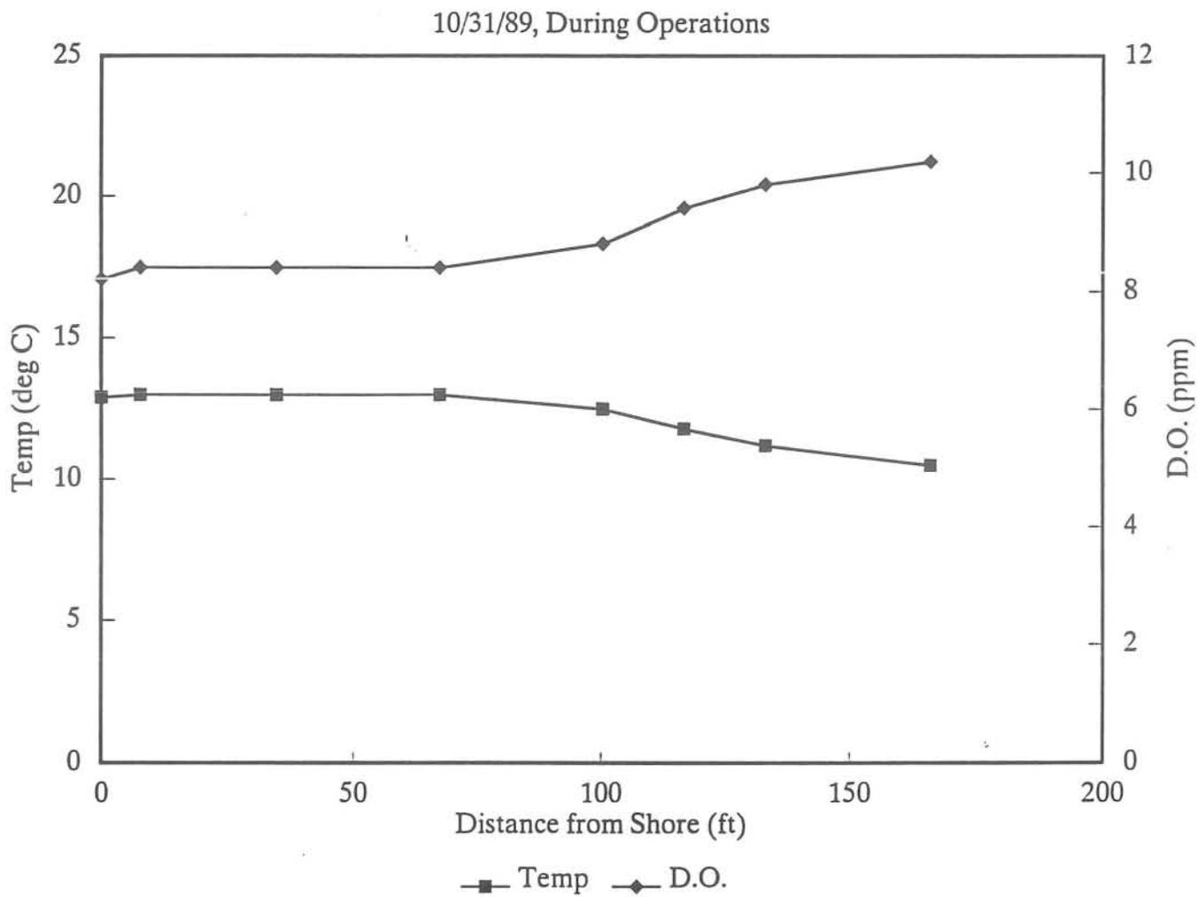
Figure 3-51. Cross-sectional profile for water temperature and dissolved oxygen (D.O.) concentrations 1000 feet below Deep Creek Project tailrace, September 19, 1989.
