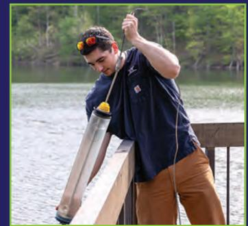
Using a special meter attached to the Kemmerer bottle, analysts can take readings at the source. They measure pH balance, total dissolved solids and other possible contaminants. Then, they pack about a liter’s worth of water into a cooler and rush it to the testing center at either the Ashburton or Montebello water filtration plants, where water is tested for potentially harmful bacteria.
