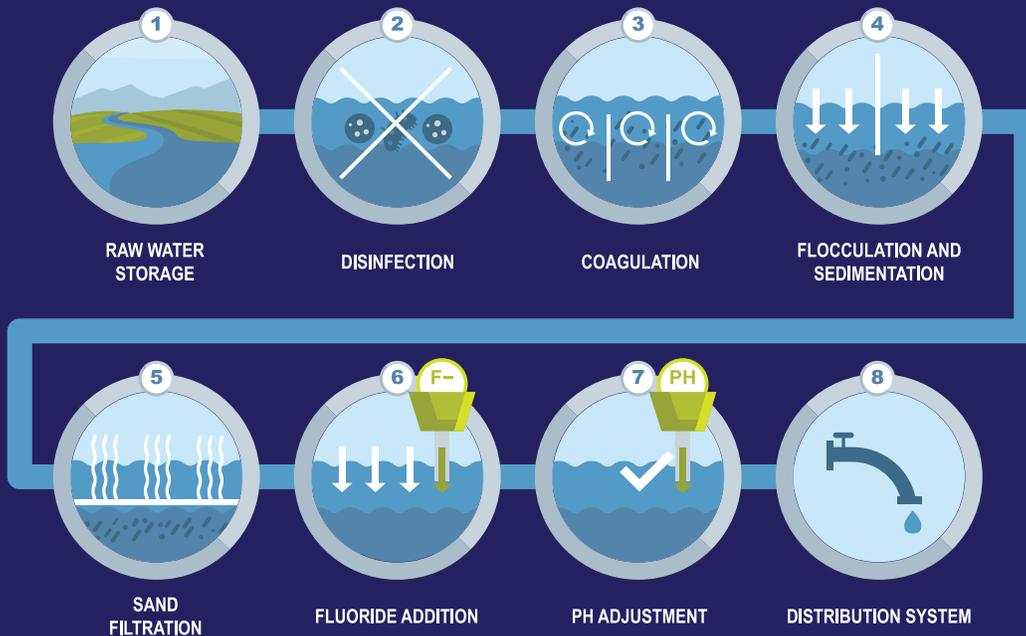
**Step 1: Raw Water Storage** – Raw water is stored at one of three City-owned reservoirs – Loch Raven and Prettyboy Reservoirs in Baltimore County and Liberty Reservoir in Carroll County. The water is conveyed through tunnels and pipes from the reservoirs to our treatment plants.
