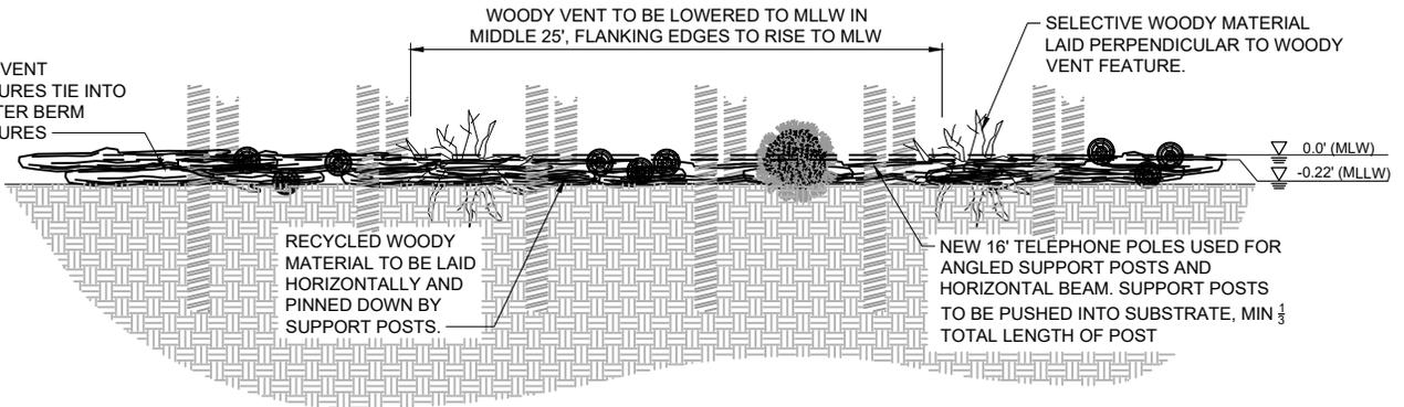
WOODY VENT TO BE LOWERED TO MLLW IN MIDDLE 25', FLANKING EDGES TO RISE TO MLW
