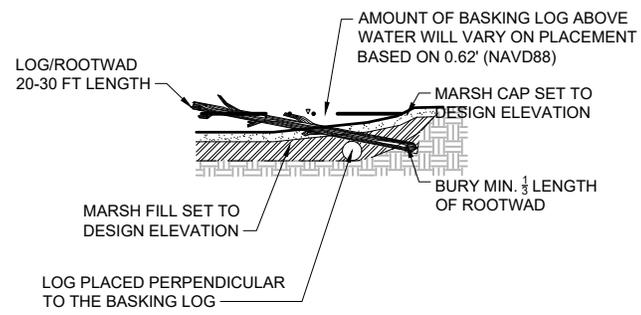
**C1** SECTION - BASKING LOG WITH ANCHOR PARTIALLY BURIED
