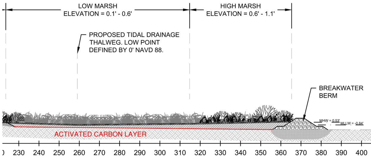
**Figure 2.** Schematic of application of thin layer of activated carbon (red line) in the areas waterside of MHW line.
