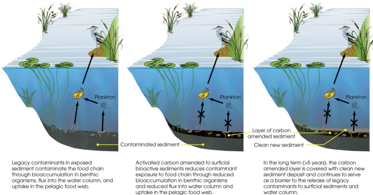
**Figure 1.** Conceptual model of how sorbent amendment of sediment reduces contaminant exposure pathways of benthic organism accumulation and flux from the sediment bed. (Ghosh et al. feature article, ES&T 2011)
