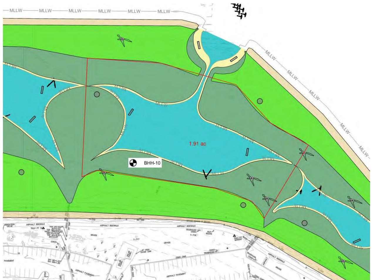
Figure 3. Schematic plan view of application of thin layer of activated carbon limits in the vicinity of BHH-10 (red line) in the areas waterside of MHW line.
