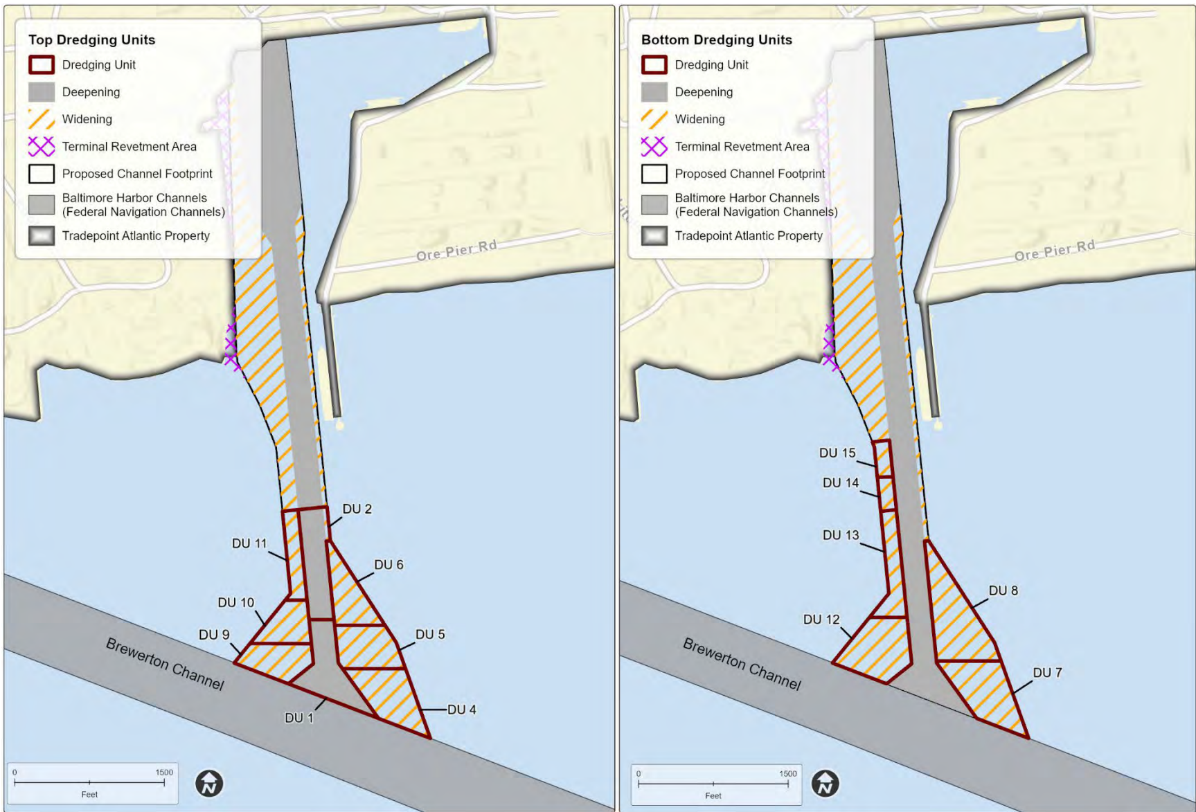
Figure 5. Sparrows Point Container Terminal: South Channel – Top and Bottom Dredging Units
