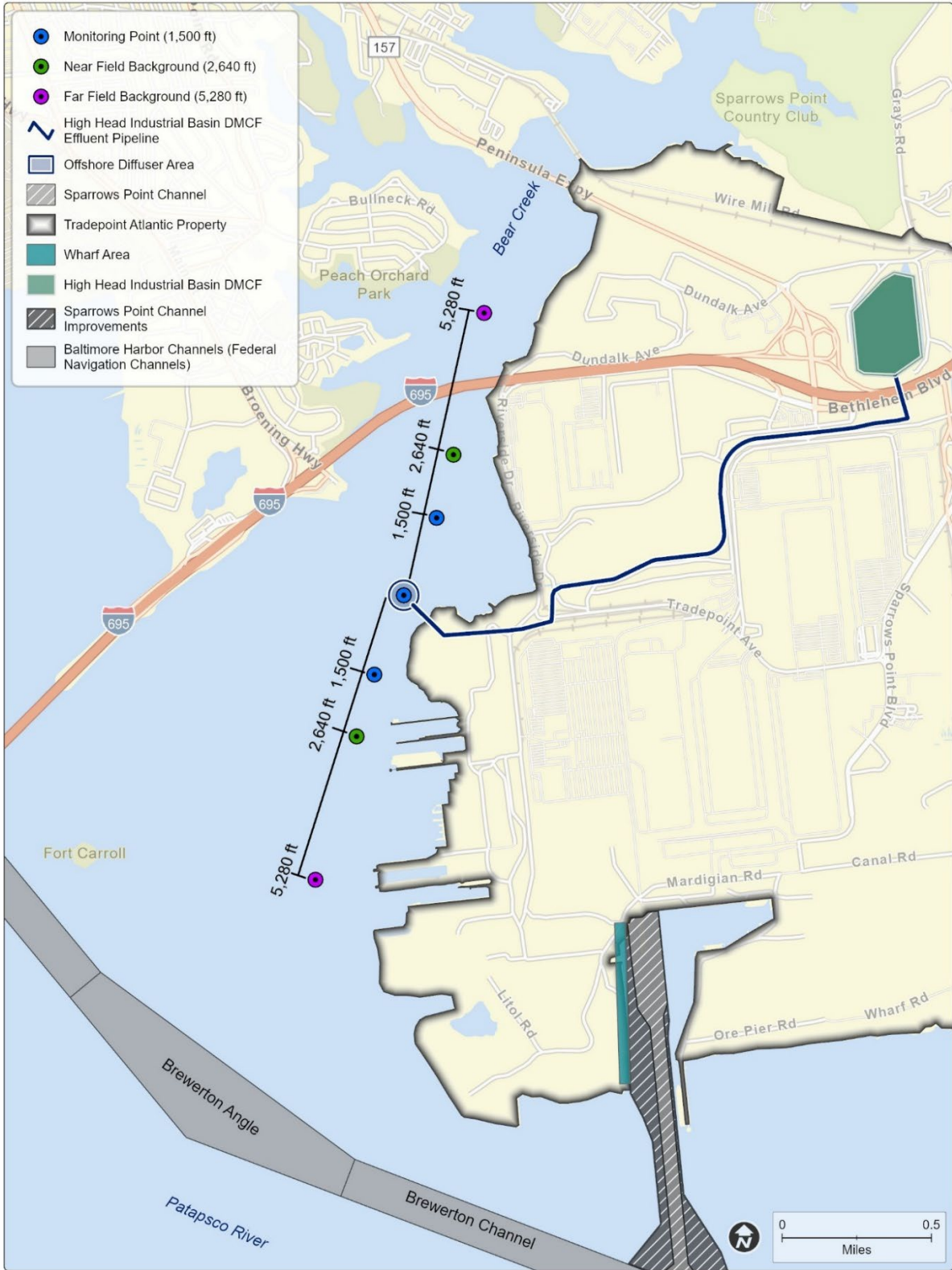
Figure 5. Sparrows Point Container Terminal: Turbidity Monitoring Locations for Temporary Diffuser Installation, Offshore West Sparrows Point Peninsula near Mouth of Bear Creek
