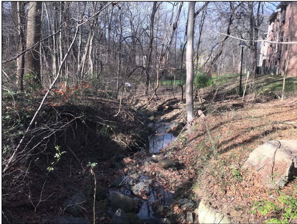
Photo 10: Reach 7, looking downstream near Cloudleap Ct, 3' actively eroding bank with minimal riparian vegetation.
