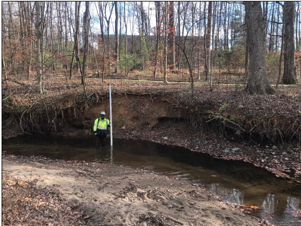
Photo 22: Reach 15B, looking upstream near Oakland Mills Rd, 9' actively eroding bank undercutting large tree
