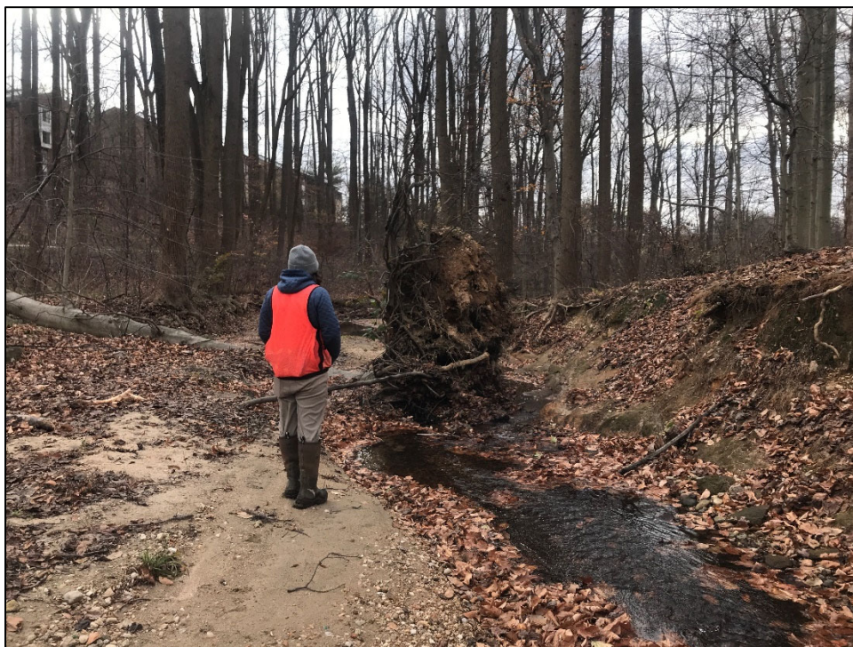
Photo 6: Reach 3B, looking downstream towards Lamb Skin Ln, 4' actively eroding bank with fallen tree.
