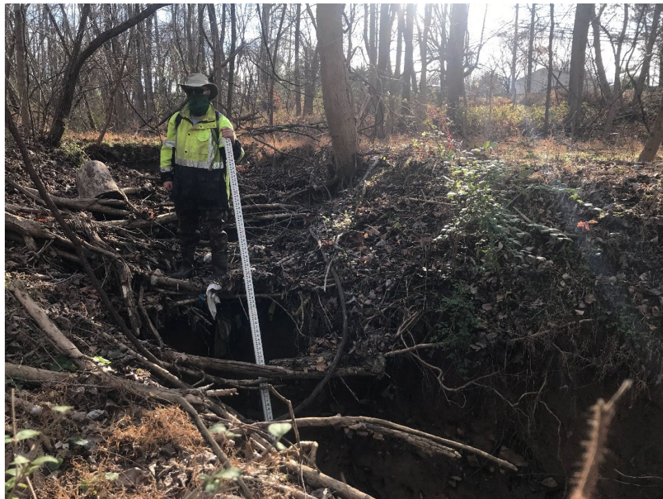
Photo 28: Reach 20, looking upstream near Oakland Mills Rd, 9' head cut and actively eroding banks.
