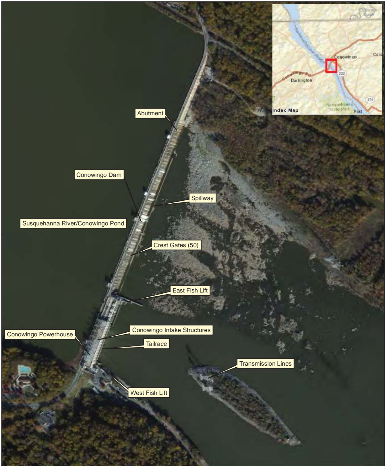
Figure 2.1.1-1: Conowingo Hydroelectric Project Major Project Facilities
