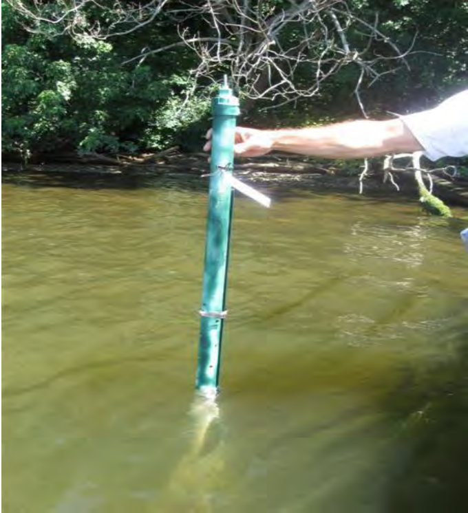
FIGURE 3.3-1. WATER LEVEL DATA LOGGER INSTALLED IN A PVC STILLING WELL.
