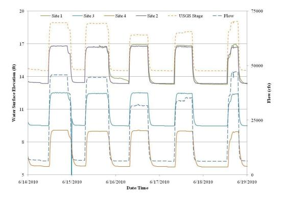
FIGURE 4.1-3: RATING CURVE COMPARING MEASURED DOWNSTREAM WATER SURFACE ELEVATIONS TO USGS GAGE FLOWS
