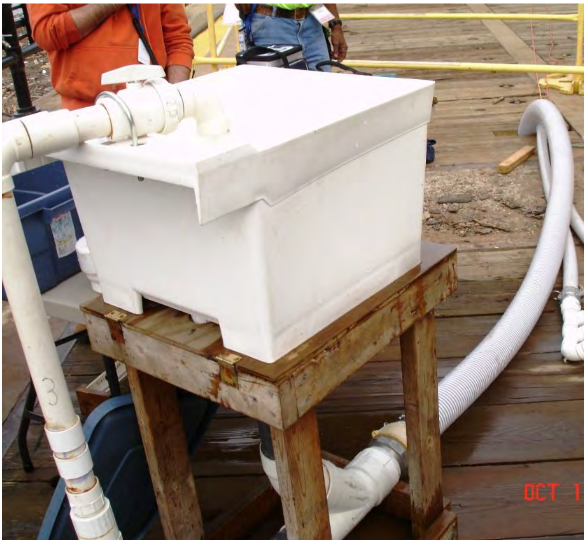
FIGURE 2.5-4: INDUCTION SYSTEM WITH DISCHARGE HOSE.
