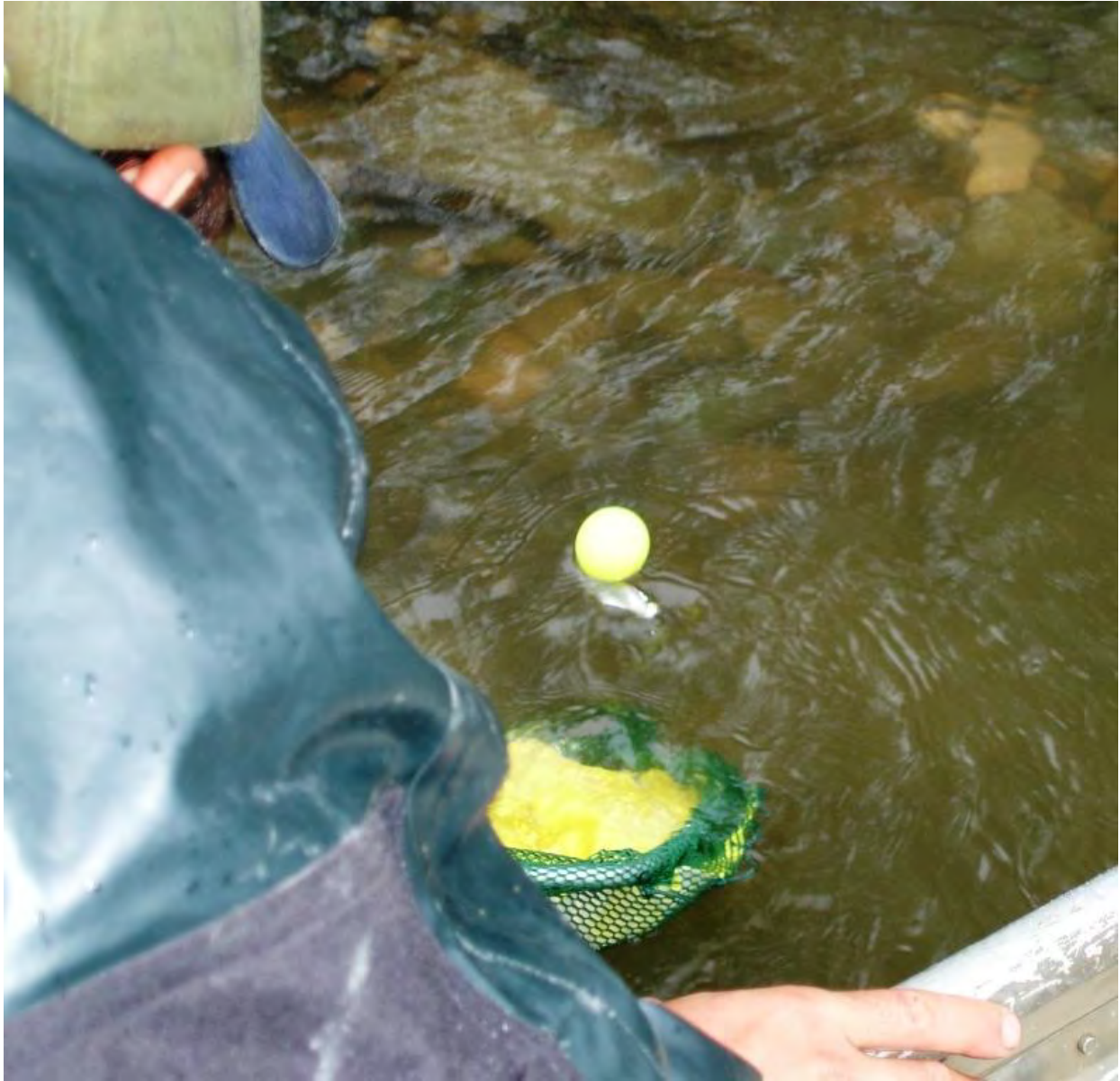
FIGURE 2.6-1: POST-PASSAGE BUOYED JUVENILE AMERICAN SHAD RETRIEVED BY WATER SANCTUARY NET OR WATER BRAILER.
