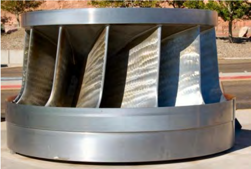
FIGURE 2.1-1: FRANCIS (TOP) AND KAPLAN/MIX-FLOW (BOTTOM) TURBINE TYPES AT CONOWINGO STATION.
