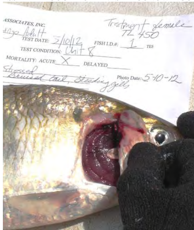
FIGURE 3.3-1: EXAMPLES OF DOMINANT INJURY TYPES OBSERVED ON ADULT AMERICAN SHAD PASSED THROUGH TURBINES AT CONOWINGO PROJECT, MAY 2012.
