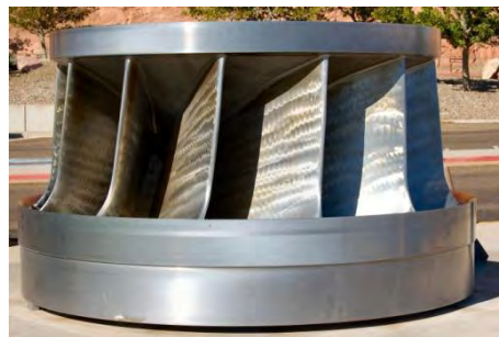
Clear picture of a typical Francis runner.
