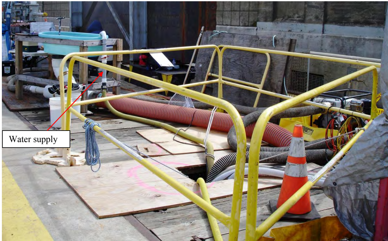
FIGURE 2.4-3: INDUCTION SYSTEM WITH DISCHARGE HOSE LOCATED ON DOWNSTREAM SIDE OF TRASH RACK.
