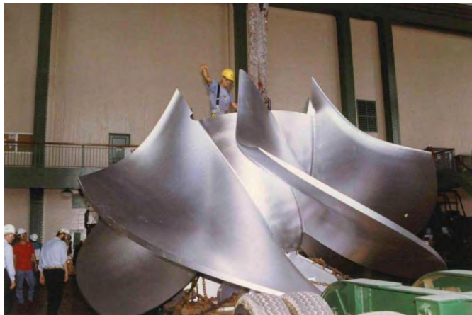
Photograph of a Kaplan runner at the Conowingo Project.
