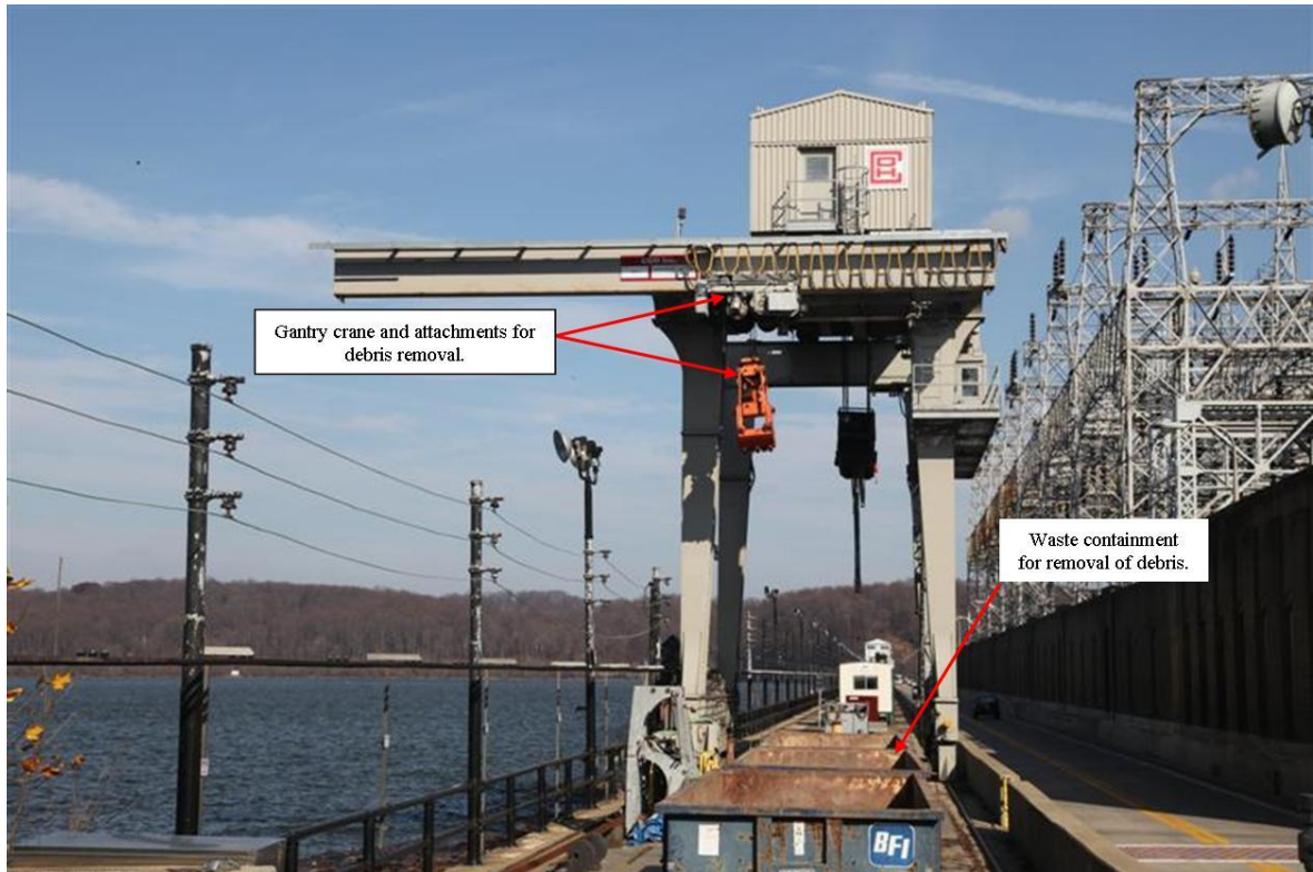
FIGURE 4.4.1-1: DEBRIS REMOVAL EQUIPMENT USED AT CONOWINGO DAM
