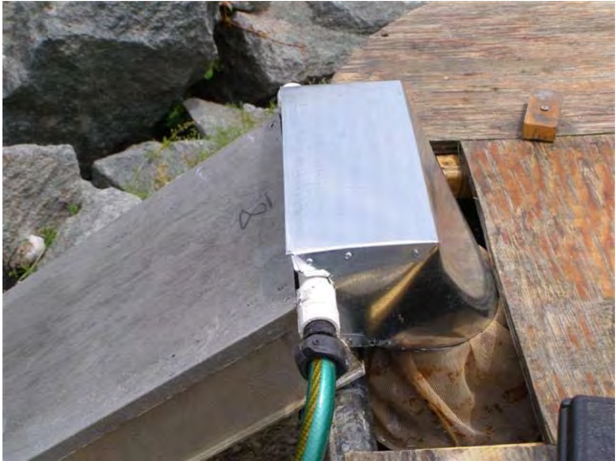
Figure 3. The cable tray emptying into a collection bag in a holding tank.
