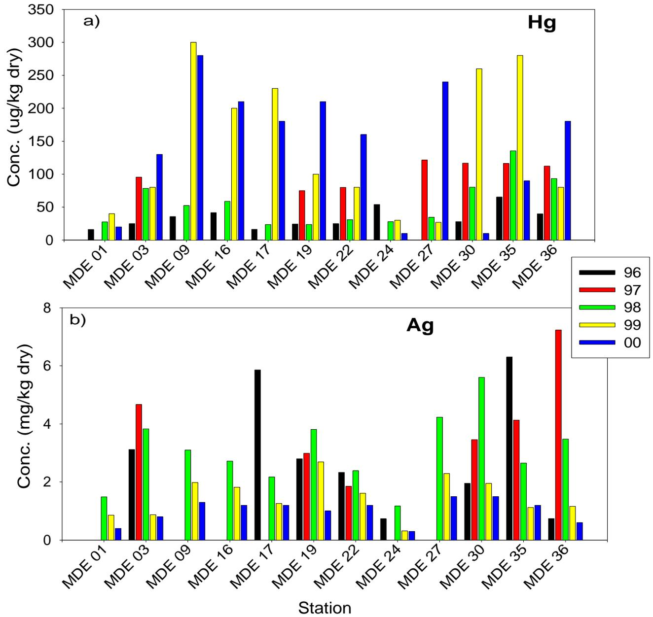
**Figure 30: Comparison of sediment mercury and silver concentrations for fall sampling for the last five years of measurement.**
