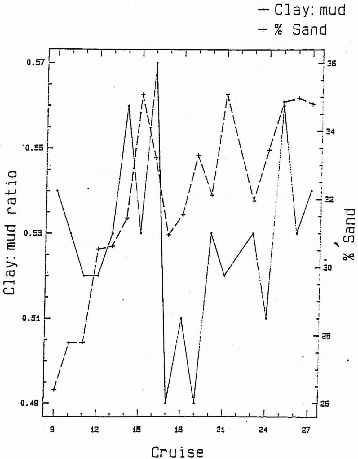
Figure 1-4: Average percent sand and clay:mud ratios, based on 24 continuously monitored stations, for all post-construction cruises through the eleventh year.
