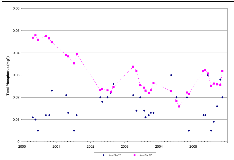
Figure D-6: Liberty Reservoir BCDPW Station NPA0059 Bottom Observed and Simulated (Calibration) TP Concentrations on Sampling Dates
