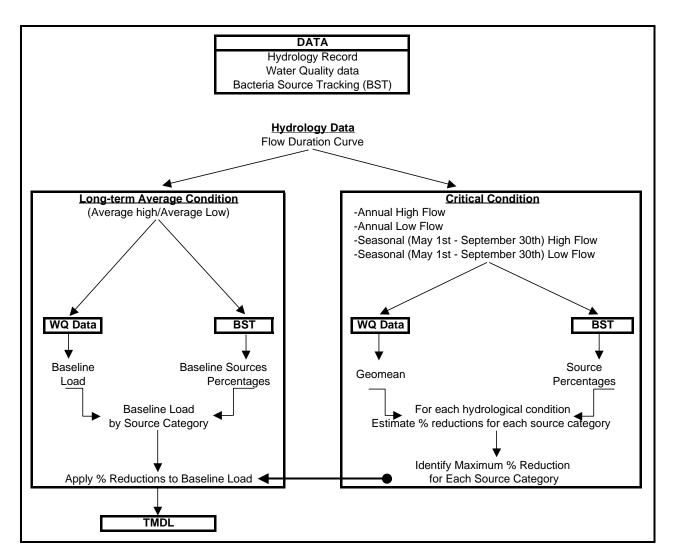
Figure 4.2.1: Diagram of Non-tidal Bacteria TMDL Analysis Framework
