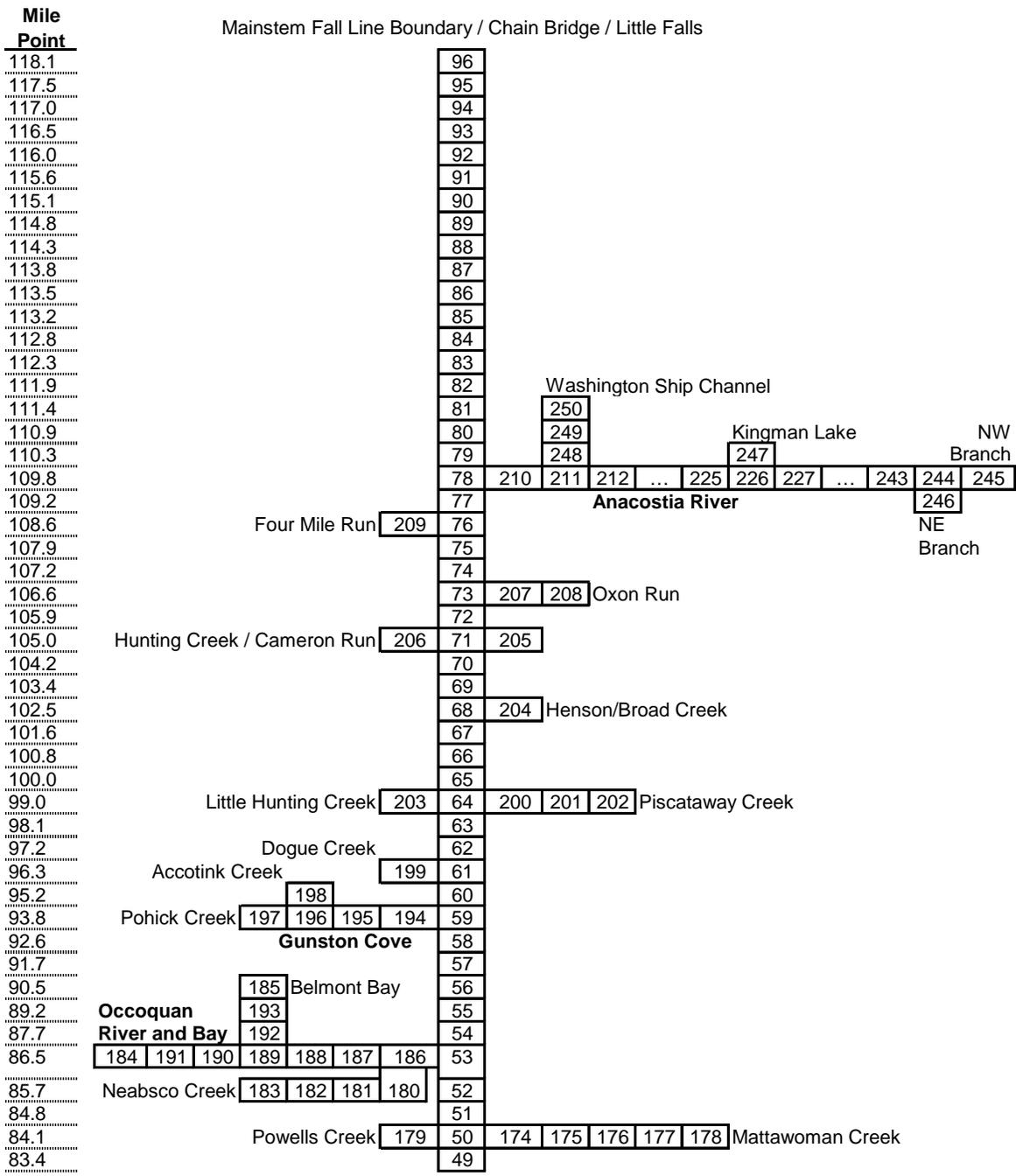
**Figure 35. Potomac Estuary POTPCB Salinity Model Segment Schematic**
