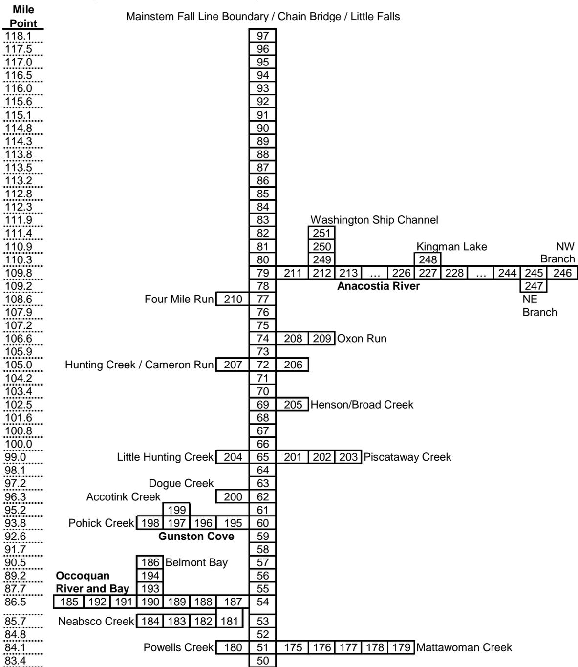
Figure 14. Potomac Estuary DYNHYD5 Model Junction Schematic
