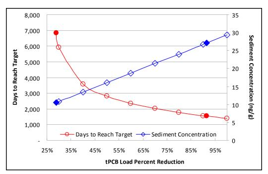
Figure F-1: Response Time (Days) to Reach the tPCB Water Column TMDL endpoint and tPCB Sediment Concentrations for Load Reductions from 29% to 100% (Solid data points represent 29% and 91.5% Reduction Scenarios)
