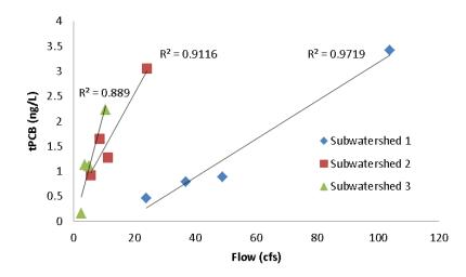
Figure C-3: Regression between PCB Concentrations and the Associated Flows of the Three Subwatersheds
