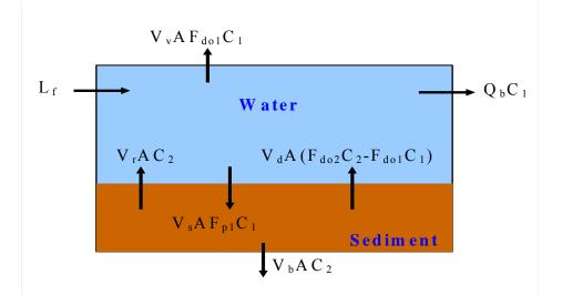
Figure D-1: Schematic Diagram of the Numerical Model and PCB Budget
