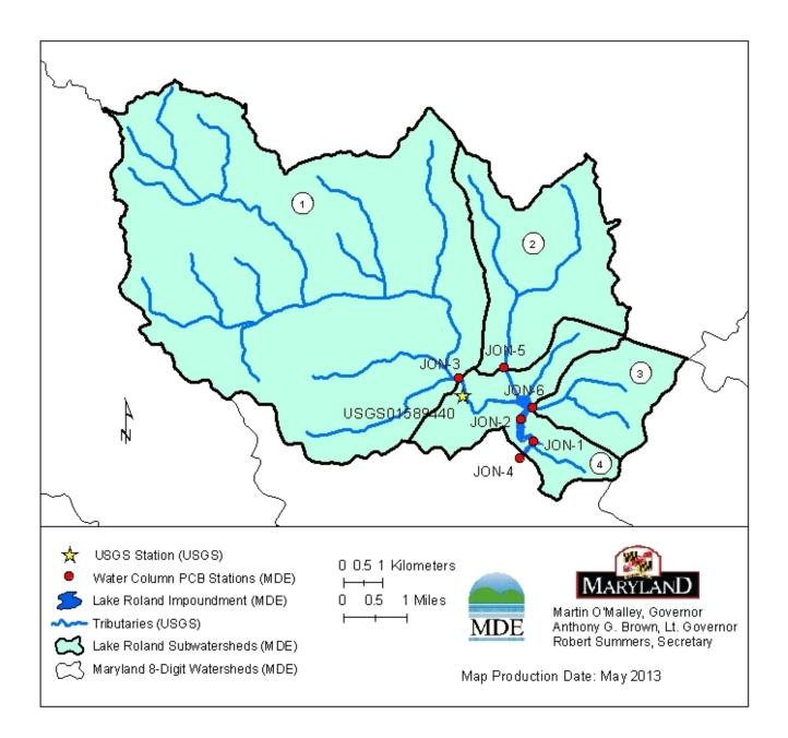
Figure C-1: The Locations of Watershed PCB Measurement Stations and the USGS Station, and the Delineation of Subwatersheds
