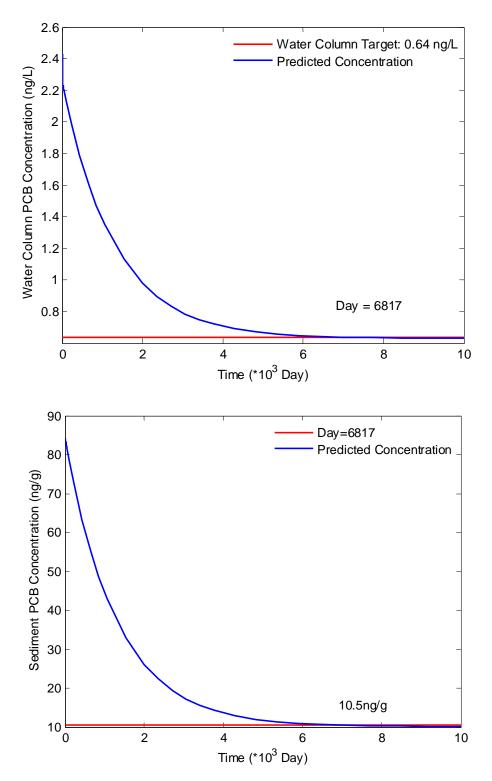
Figure 10: Change of Average Water Column and Bottom Sediment tPCB Concentrations over Time within the Lake Roland Impoundment Assuming a 29% Load Reduction
