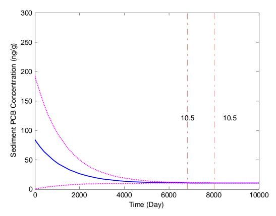
**Note**: The dashed red lines in the sediment graph represent what the sediment concentrations will be within the impoundment when the water column TMDL endpoint concentration is achieved in the 2 different scenarios (*i.e.*, mean and upper CIs). As in the lower CI scenario, the water column concentration meets the endpoint from the very beginning, no dash line is generated.
