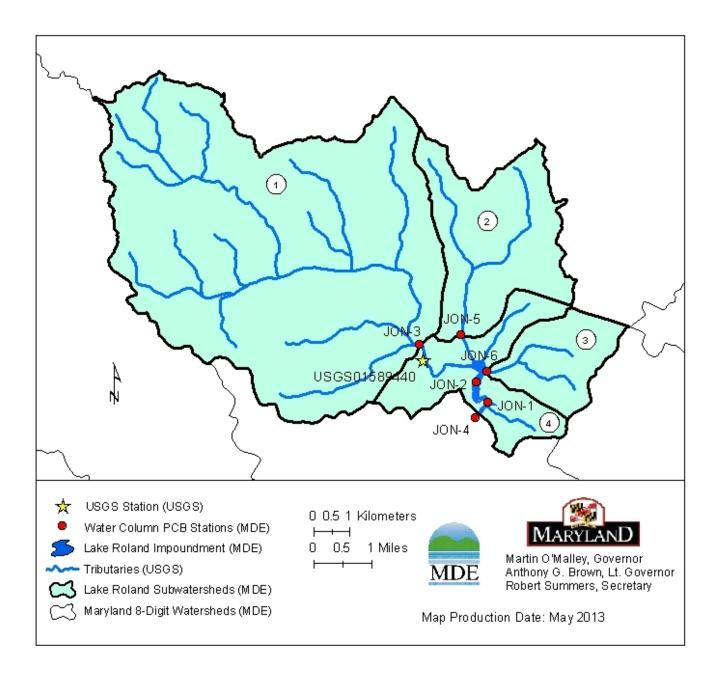
Figure 4: The Locations of Watershed PCB Measurement Stations and the USGS Station, and the Delineation of Subwatersheds
