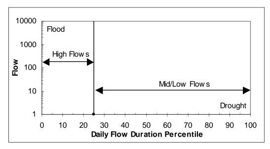
Figure 2.3.1: Conceptual Diagram of Flow Duration Zones
