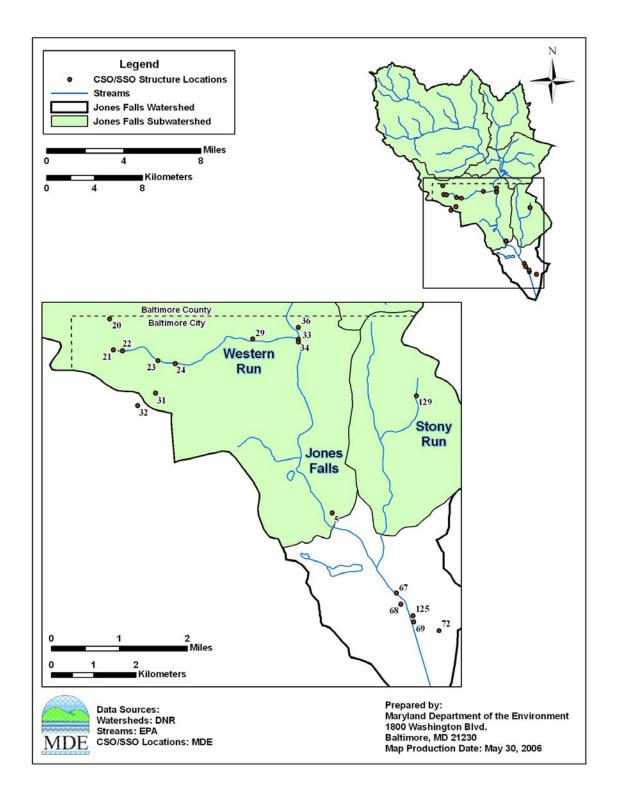
Figure 2.4.3: Sanitary and Combined Sewer Overflows Structures in the Jones Falls Watershed
