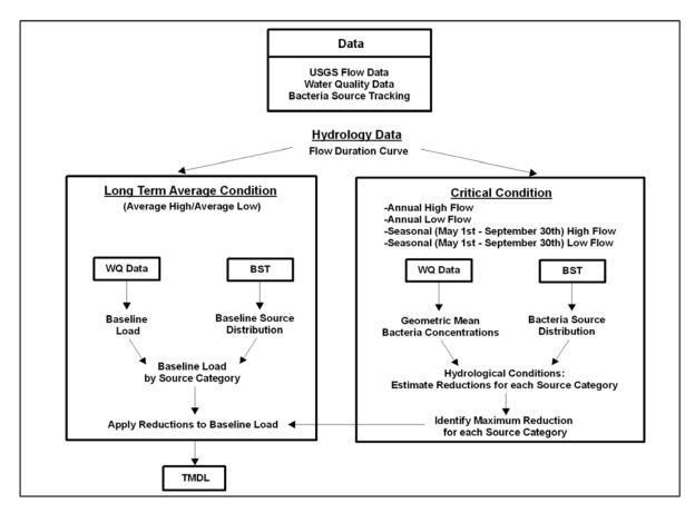
Figure 4.2.1: Diagram of Non-tidal Bacteria TMDL Analysis Framework
