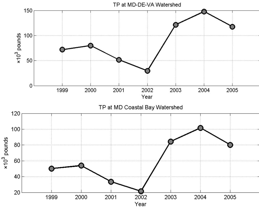
**Figure 23. Predicted annual loads of total phosphorus in the MD-DE-VA Coastal Bays watershed and in Maryland's portion of the Coastal Bays watershed.**
