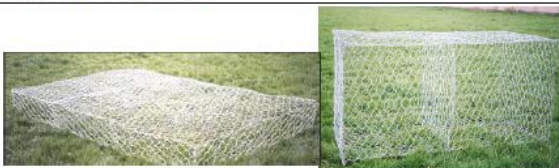
Figure 5-2.—Typical unfilled gabion basket on left and mattress on right. Each is formed with compartments to minimize rock movement within the gabion and deformation of the overall structure. Hexagonal woven steel wire mesh gabions are shown (Reclamation, courtesy of Chris Ellis).
