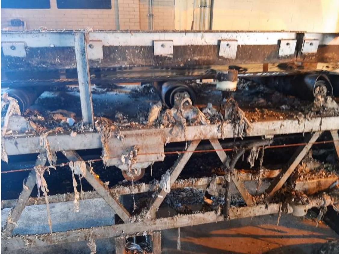
6/29/22 trash clogging conveyor belt. This area should be routinely cleaned of trash and maintained in a manner that promotes effective functioning of the system. The permittee must improve operating practices in this area.
