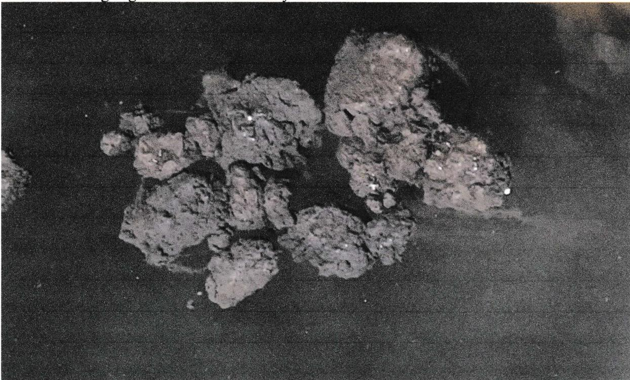
4/22/22 Floating solids in clarifier 14A similar to floating solids in the contact chambers
