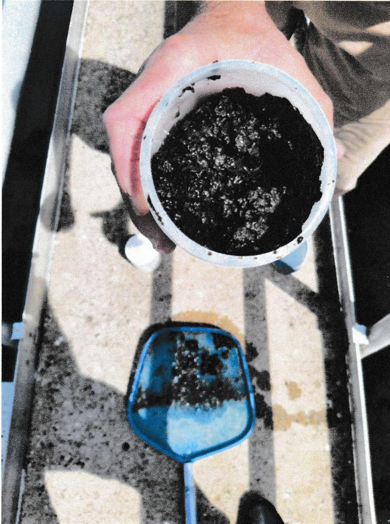
4/22/22 sample of the floating solids at the contact chamber.
