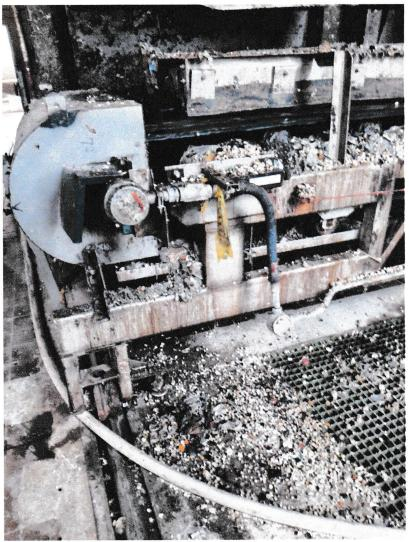
4/6/22 Trash overflowing the belt transport system
