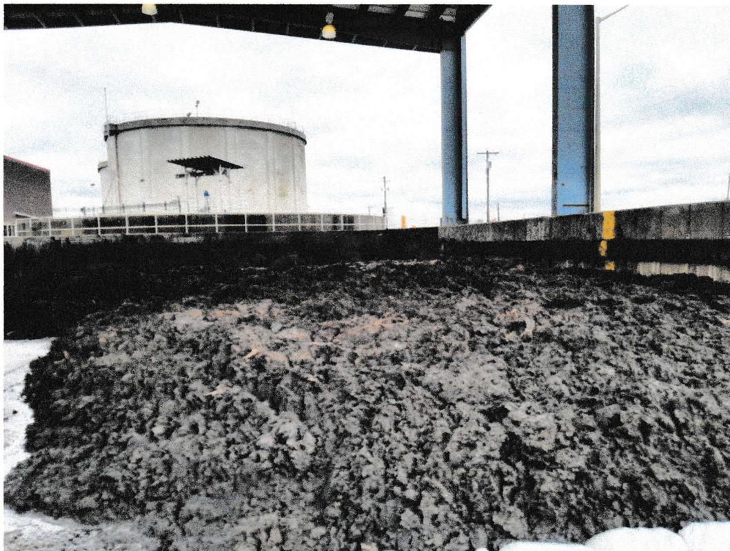
4/6/22 stored untreated sewage sludge. Sludge should have been placed to the rear of the yellow marking on the right side of the picture.
