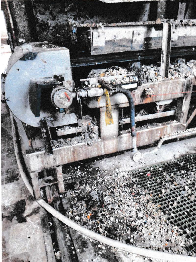
4/6/22 Trash overflowing the belt transport system
