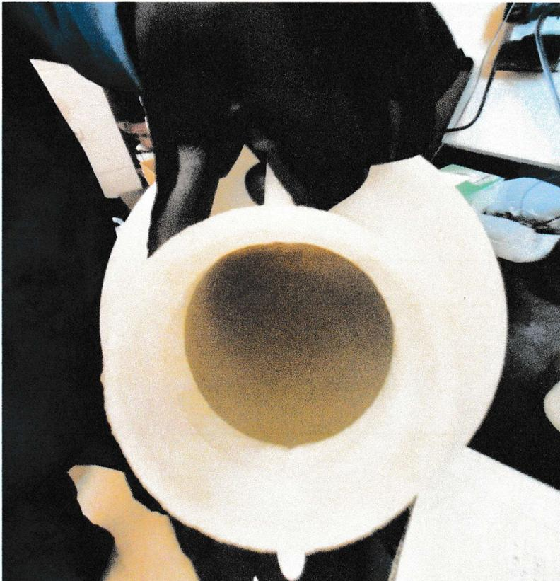
4/6/22 Final effluent composite sample dark opaque grey with particulates
