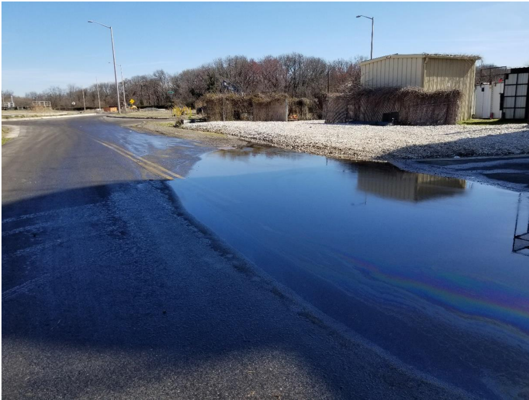
Picture 3: An oily sheen and green-ish color were observed in the flow water along the flow path from the pelletech building towards the dried sludge loading building.
