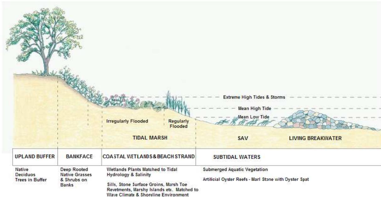
**Figure 3.6 Schematic of living shoreline restoration**
