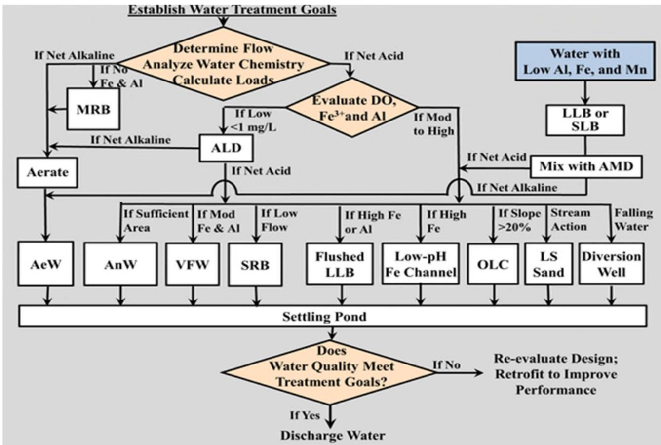
Key: MRB- Manganese Removal Bed, ALD – Anoxic Limestone Drain, AeW – Aerobic Wetland, AnW – Anoxic Wetland, VFW – Vertical Flow Wetland, SRB – Sulfate Reducing Bioreactor, LLB – Limestone Leached, OLC – Open Limestone Channel, LS – Limestone, SLB – Slag Leached
