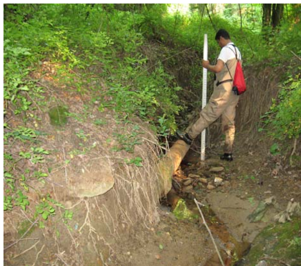
Figures 18A & B: Exposed utility and erosion in SR-08-02-01
