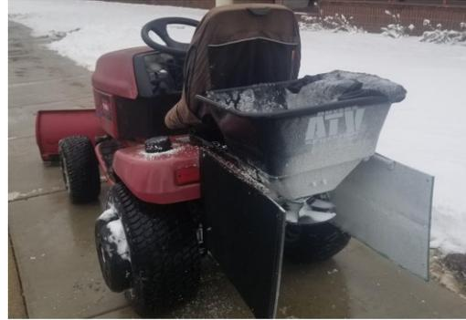
*Figure 39. Combination sidewalk plow and salt spreader outfitted with deflection shields. Image from Jason Swope.*
