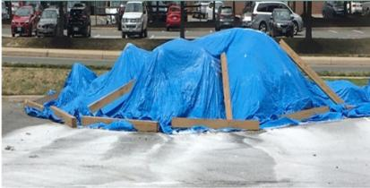
Figure 42. Improper salt storage due to lack of containment Image from [Fairfax County, Va.](#)
