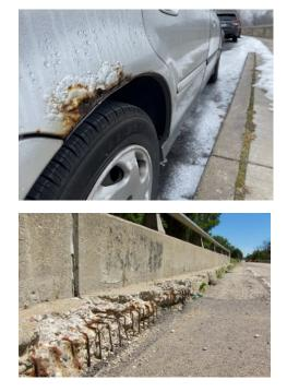
Figure 10. Example of car (top) and metal reinforced concrete (bottom) corrosion. Top image by ICPRB. Bottom image from McHenry County courtesy of Scott Kuykendall.
