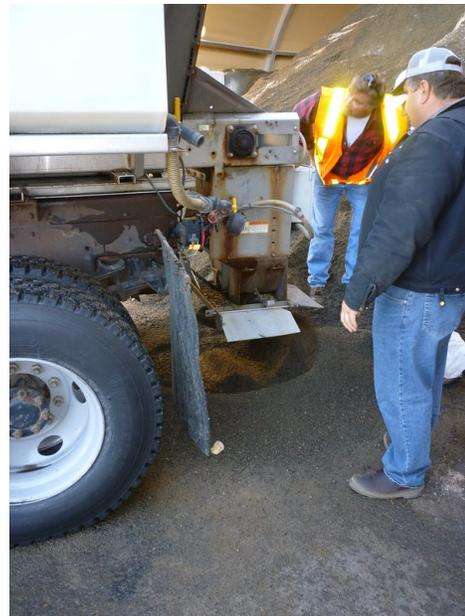
Figure 90. Sand/salt spreader on the snowplow. Image by WSDOT from Flickr.
