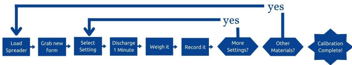
Figure 87. Steps for calibrating an auger or conveyor system. Adapted from MPCA training manual [1].
