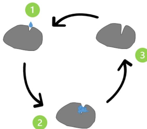
Figure 11. Example of the freeze/thaw cycle. (1) Water enters small cracks in rocks, concrete, and other impervious surfaces. (2) Water freezes, increasing pressure on the surrounding area leading to (3) The extra pressure causes the cracks to enlarge. Image from ICPRB.
