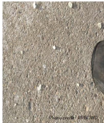
Figure 4-15 The deicer should have space between the granules.
