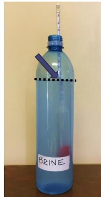
Figure 60. Example of hydrometer in salt brine. Notice, the percent concentration of the salt in the solution is where the dotted line meets the water. Image from [2].
