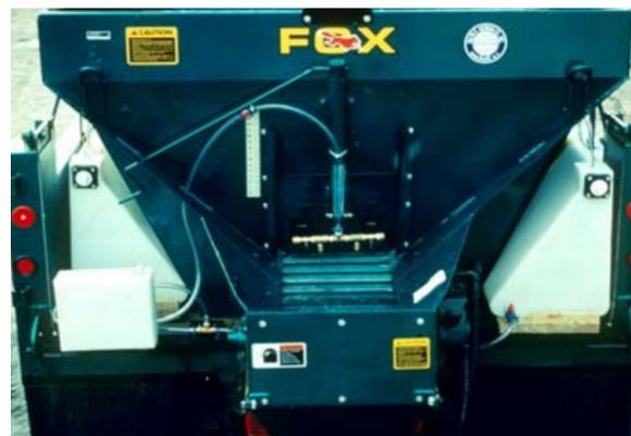
Figure 65. Example of a pre-wetting machinery on a winter maintenance truck. Image from NHDES BMP PreWetting.
