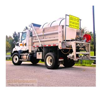
Figure 56. Liquid deicing equipment being used for ant-icing prior to a winter storm. Image by Seth Granville from Flickr Commons.
