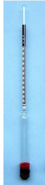
Figure 59. Example of a hydrometer. Image Qlaz from Wikimedia.
