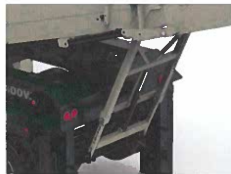
Hydraulic height adjustment on discharge conveyor.
