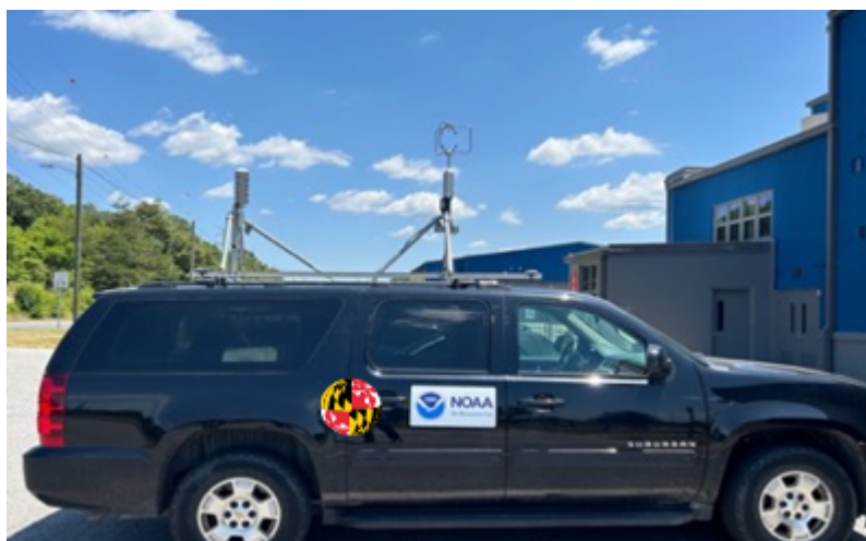
Figure 30. NOAA's ARC or Air Resources Car with roof rack supporting a sonic anemometer and inlets for trace gases and aerosols (forward) and other meteorological sensors (aft).
