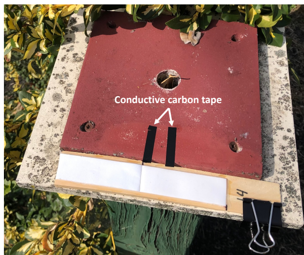
Figure 11. Passive ambient particle accumulation (PAPA) sampling at Location C, a residential sampling site in Curtis Bay, MD (October 26, 2023 to October 29, 2023). Note the two conductive carbon tape segments with co-located white tape collector to visualize settled dust.
