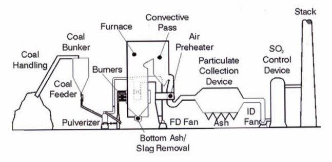
The CCBs currently produced and used are a result of the combustion of pulverized coal.
