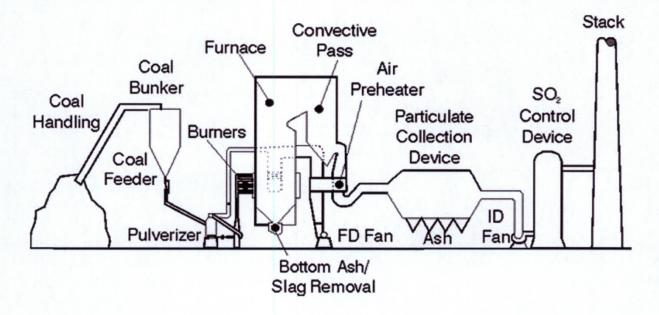
The CCBs currently produced and used are a result of the combustion of pulverized coal.
