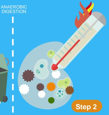
Collected packaged food waste is "depacked" and turned into a slurry. The slurry is heated to ~104° F. This allows the microorganisms to begin creating biogas.
