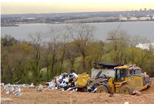
Figure 1-3 Loader-Assisted Grab Sampling of Inbound MSW Sampling
