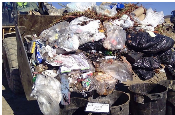
Figure 1-3 Loader-Assisted Grab Sampling of Inbound MSW Sampling
