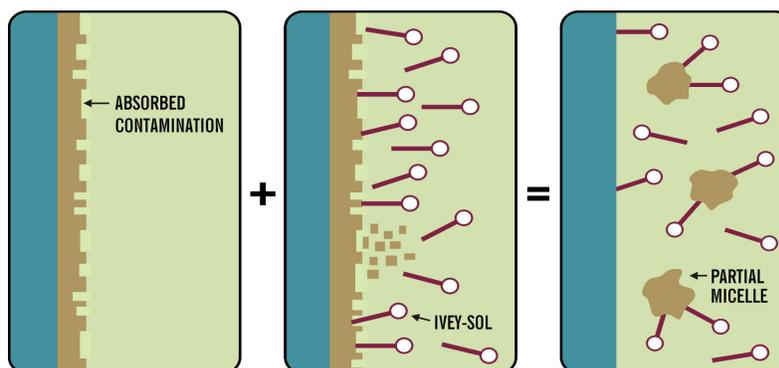
**Ivey-sol<sup>®</sup> shown desorbing contamination off a surface. Once liberated the desorbed contaminants have increased 'availability' for improving the associated in-situ and/or ex-situ remediation method being employed.**
