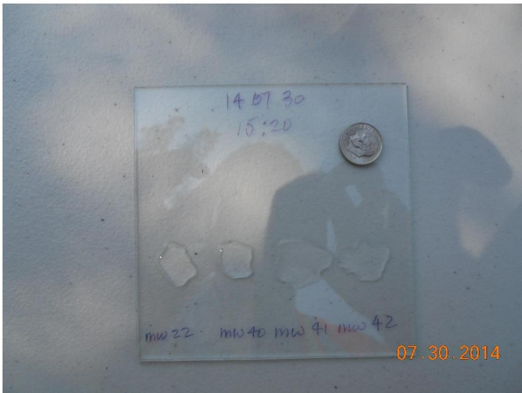
**Side View – Note the irregular shape and lack of height of droplets compared to the dime indicating general presence of surfactant.**
