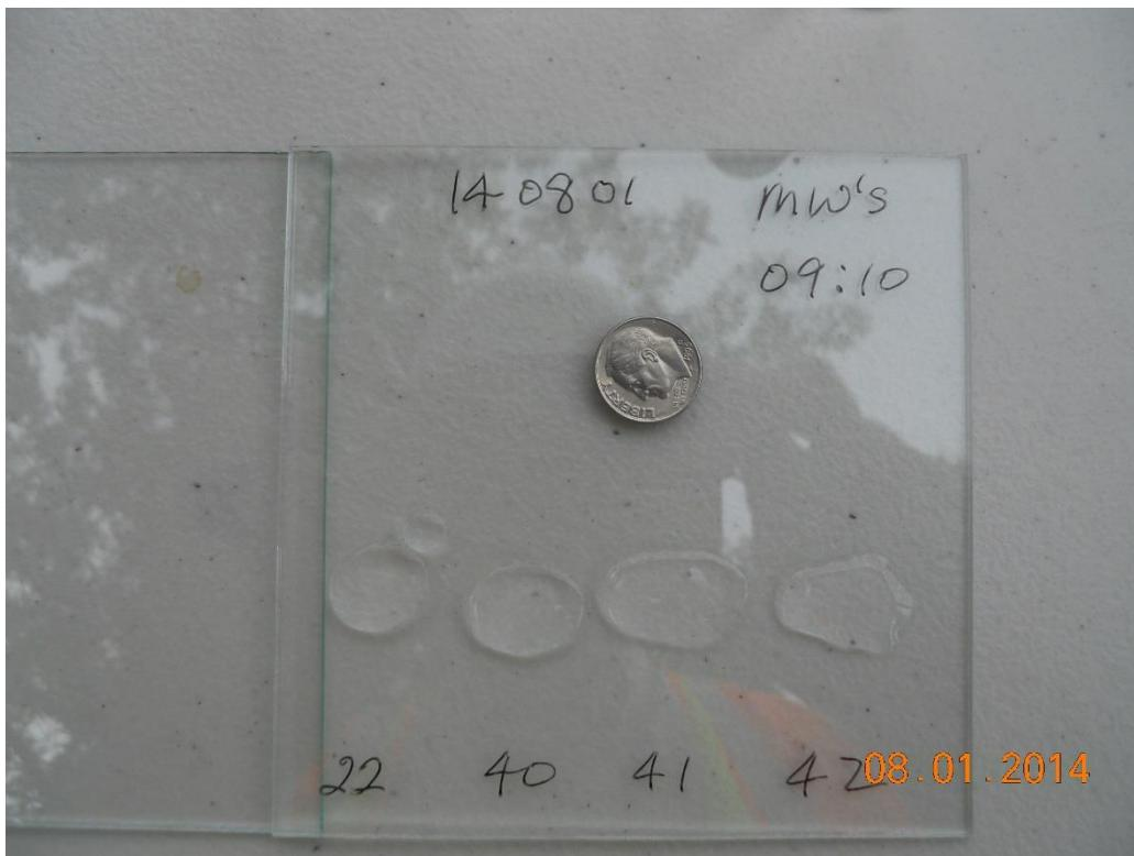
**Side View – Note droplets from MW-22 and MW-40 show uniform size and height compared to the dime indicating the general absence of surfactant while MW-41 and MW-42 droplets are relatively flat indicating the presence of surfactant.**
