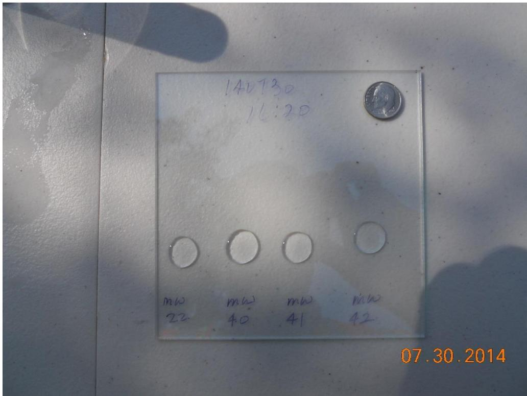
**Side View – Note uniform and comparable height of water droplets to dime indicating general absence of surfactant.**
