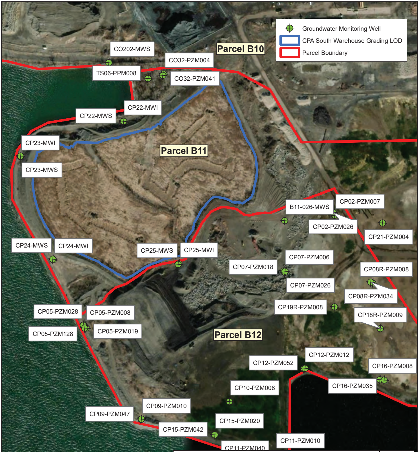
Sub-Parcel B11-1/CPA South Warehouse Groundwater Monitoring Well Locations March 17, 2023
