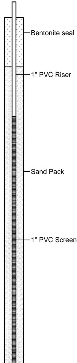
Boring terminated at 14' bgs due to water and piezometer installation.
