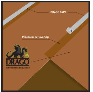
Unroll Drago Wrap over the area where the slab is to be placed. Drago Wrap should completely cover the concrete placement area. All joints/seams should be overlapped a minimum of 12 inches and taped using Drago<sup>®</sup> Tape. (Fig. 1). If additional protection is needed, install DragoTack<sup>™</sup> Tape in between the overlapped seam in combination with Drago Tape on top of the seam.
