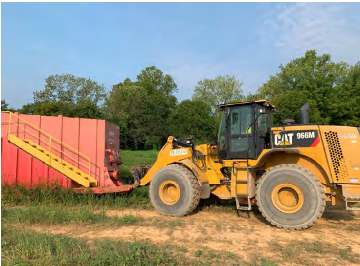
Photo 191: Rubber tire loader adjusting Tank 1 location onto flat ground to facilitate tank relocation. (August 22, 2023)
