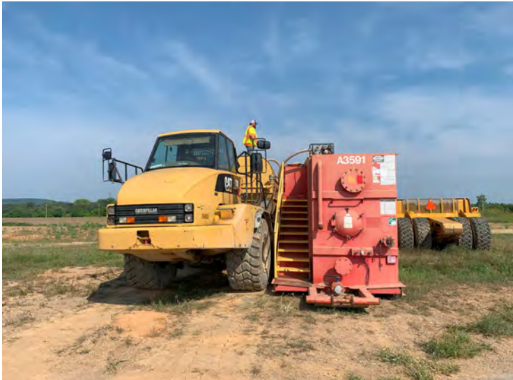
Photo 185: Pumping water from the water truck into Tank 2. (August 21, 2023)
