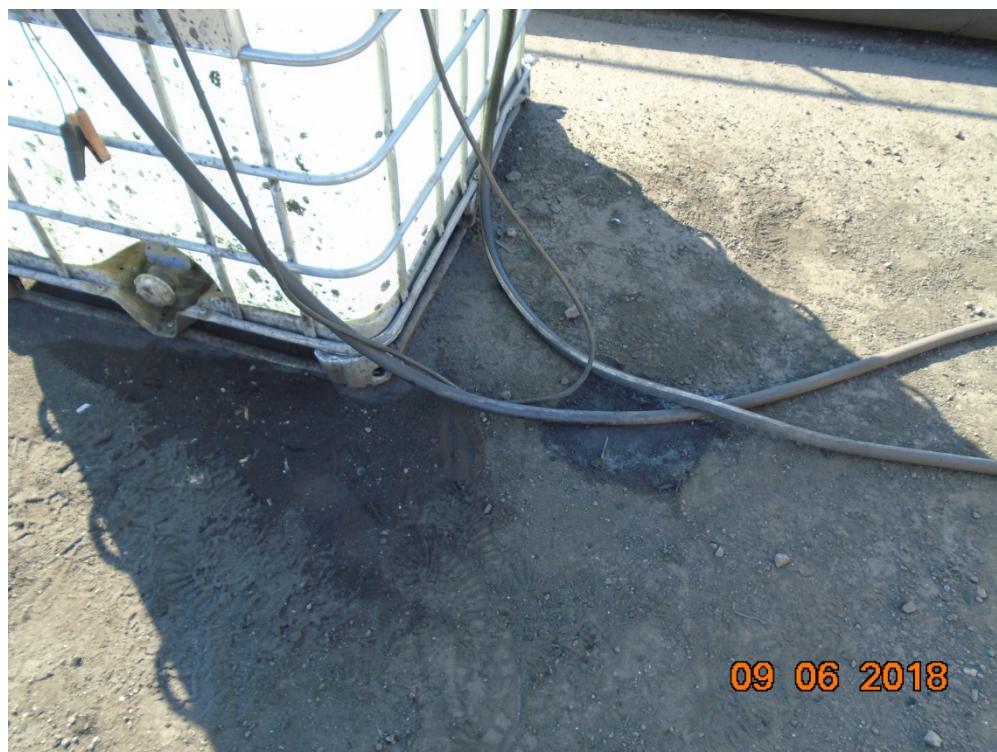
Photo 16: View of spill evidence next to the DEF Tote.
