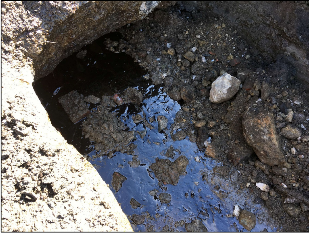
022417-3: Another view of the NAPL found in the photo above leaching out of the concrete box.
