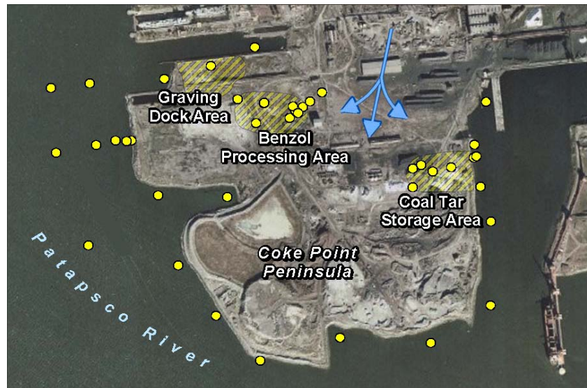
Figure 2. Sampling Locations and Areas of Concern. Yellow dots show onshore and offshore sampling locations; yellow hatching shows onshore areas of concern; blue arrows indicate direction of shallow groundwater flow.
