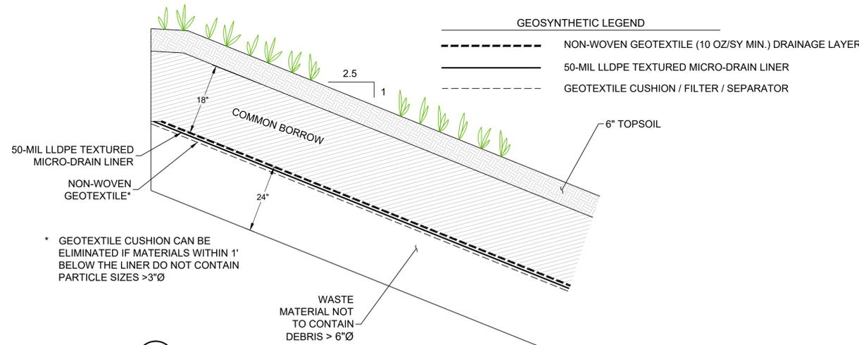
\* GEOTEXTILE CUSHION CAN BE ELIMINATED IF MATERIALS WITHIN 1' BELOW THE LINER DO NOT CONTAIN PARTICLE SIZES >3"Ø
