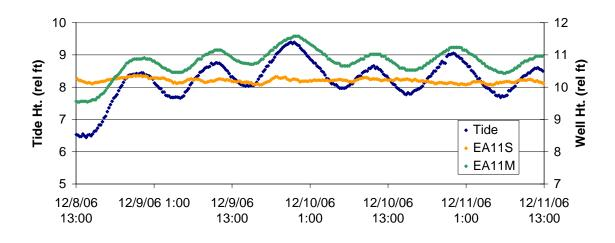
Figure 3-12. Level variation in monitoring well pair EA-11S/EA-11M compared to variations in the harbor tide.
