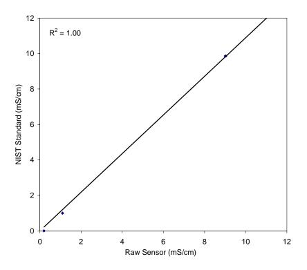
Figure 3-1. Trident probe conductivity sensor calibration.
