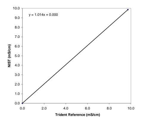
Figure 3-3. Trident reference conductivity sensor calibration.
