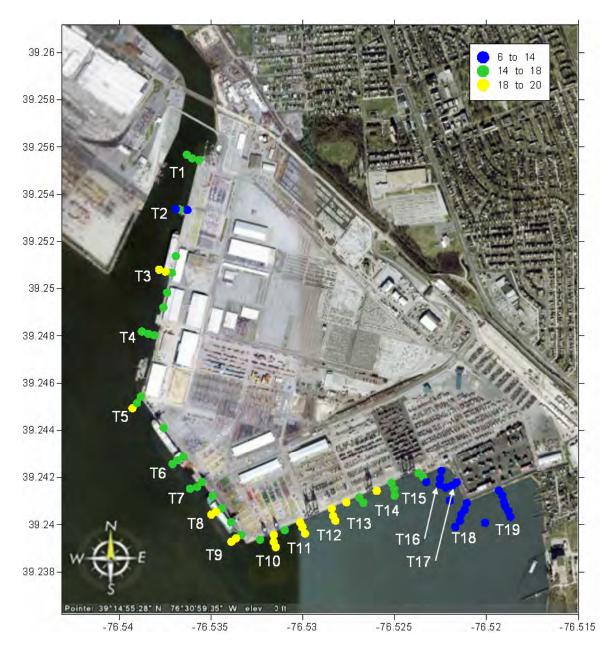
Figure 3-10. Trident reference sensor conductivity (mS/cm). Reference conductivities were measured within 1 ft of the bottom.
