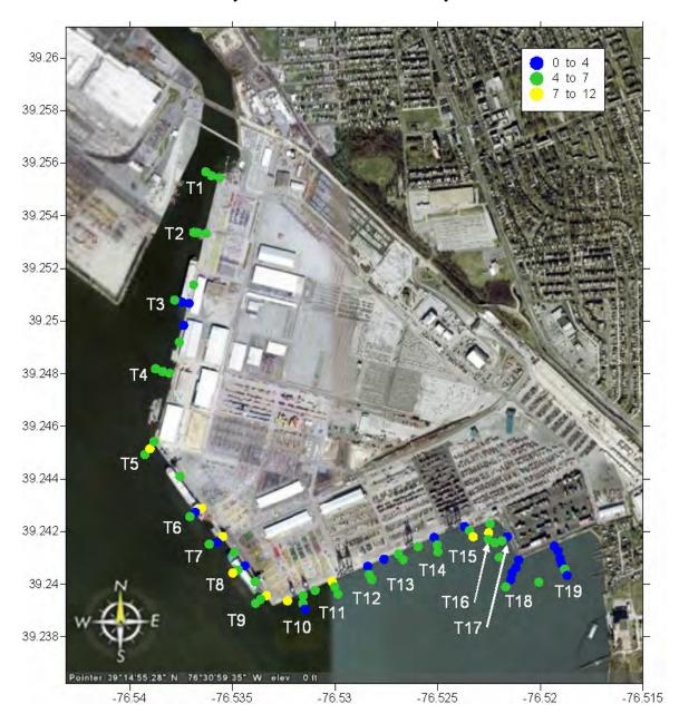
Figure 3-5. Trident subsurface conductivity distribution (mS/cm).
