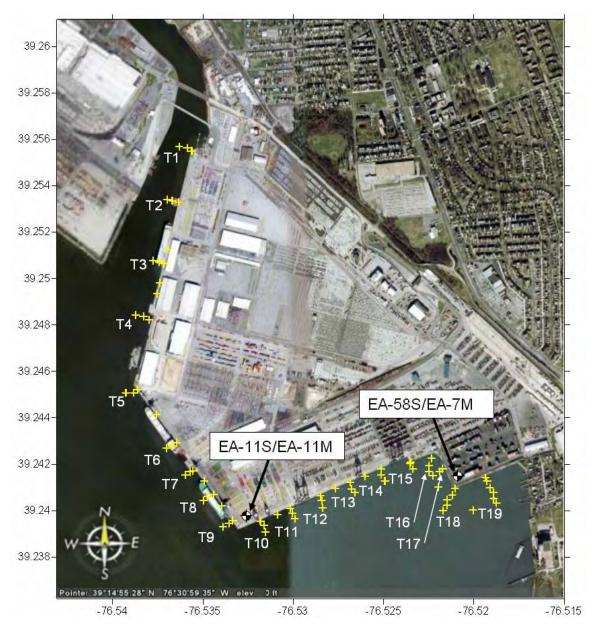
Figure 2-2. Sampling grid for the Trident Probe sensor survey offshore from DMT. Labels indicate transect numbers. Individual stations were designated A,B,C... with increasing distance from shore. Intermediate transects were designated with fractional designations based on the relative position between adjacent primary transects (e.g. T3.5).
