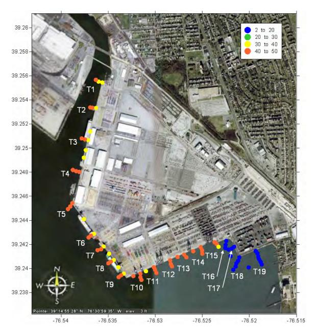
Figure 3-9. Bottom depth readings (ft) obtained during the Trident survey. Depths were measured by hand-held acoustic sounder and are not corrected for tidal variation.
