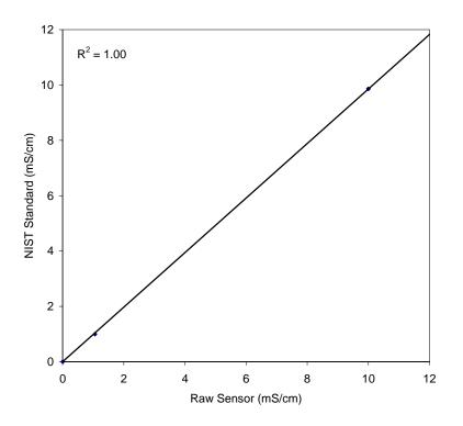
Figure 3-3. Trident reference conductivity sensor calibration.
