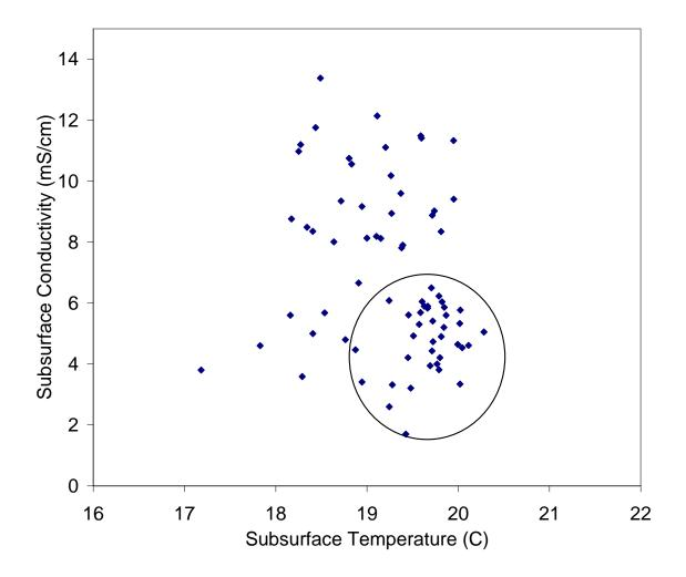
Figure 3-7. Relationship between subsurface conductivity and temperature. Circle indicates cluster of stations with relatively low conductivity and high temperature.
