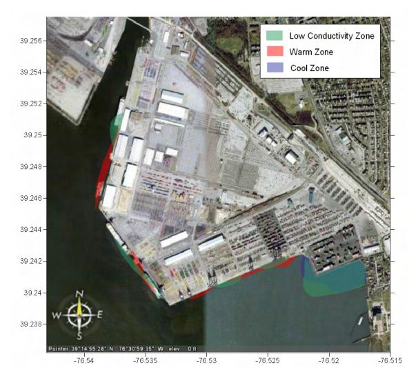
Figure 3-8. Potential discharge zones based on Trident subsurface conductivity and temperature.
