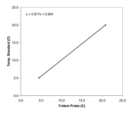
Figure 3-2. Trident probe temperature sensor calibration.
