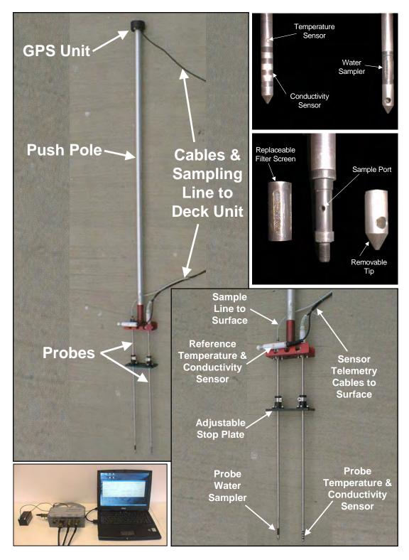
Figure 2-1. Complete Trident Probe showing sensor and water sampling probes, pushpole, GPS unit, expanded view of sensors and water sampler, and deck unit.
