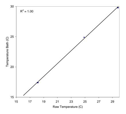
Figure 3-2. Trident probe temperature sensor calibration.
