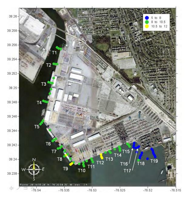
Figure 3-11. Trident reference sensor temperature (C). Reference temperatures were measured within 1 ft of the bottom.
