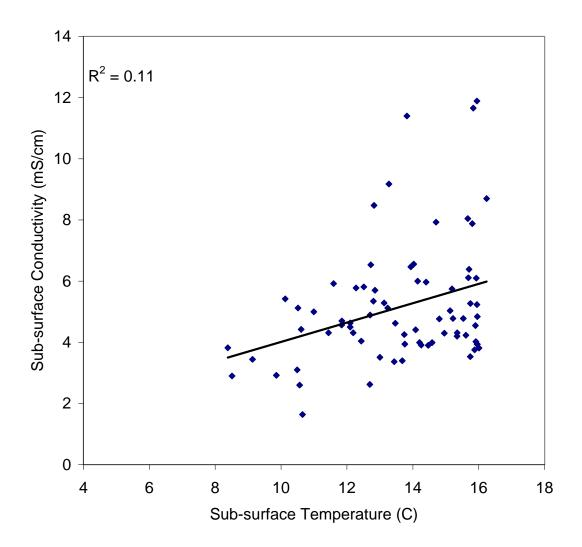
Figure 3-7. Relationship between subsurface conductivity and temperature.
