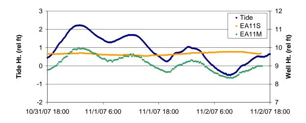
Figure 3-9. Level variation in monitoring well pair EA-11S/EA-11M compared to variations in the harbor tide.
