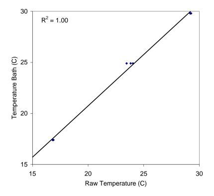
Figure 3-4. Trident reference temperature sensor calibration.
