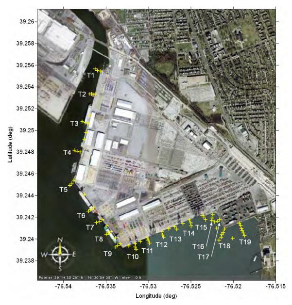
Figure 2-2. Sampling grid for the Trident Probe sensor survey offshore from DMT. Labels indicate transect numbers. Individual stations were designated 1,2,3... with increasing distance from shore. Intermediate transects were designated with fractional designations based on the relative position between adjacent primary transects (e.g. T3.5).
