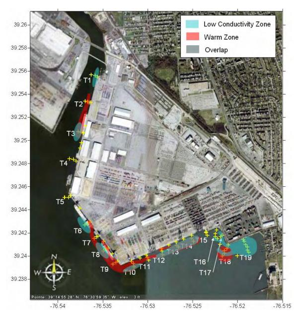
Figure 3-8. Potential discharge zones based on Trident subsurface conductivity and temperature.
