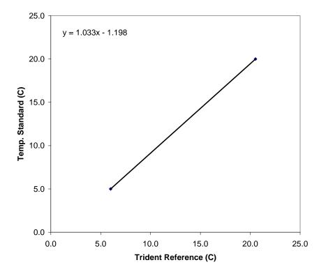
Figure 3-4. Trident reference temperature sensor calibration.
