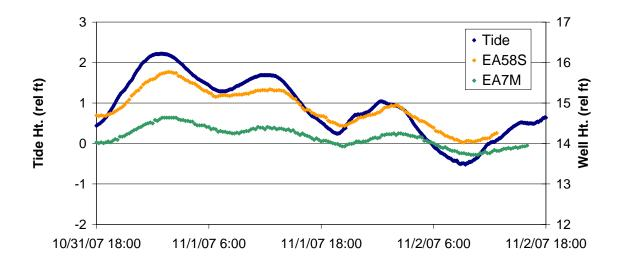
Figure 3-10. Level variation in monitoring well pair EA-58S/EA-7M compared to variations in the harbor tide.
