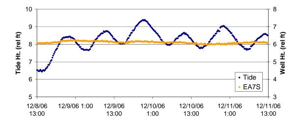
Figure 3-13. Level variation in monitoring well pair EA-7S compared to variations in the harbor tide.
