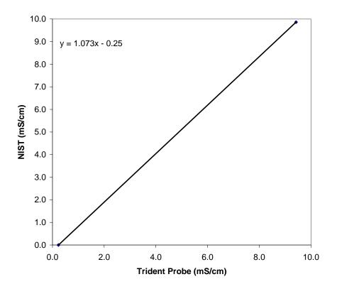
Figure 3-1. Trident probe conductivity sensor calibration.
