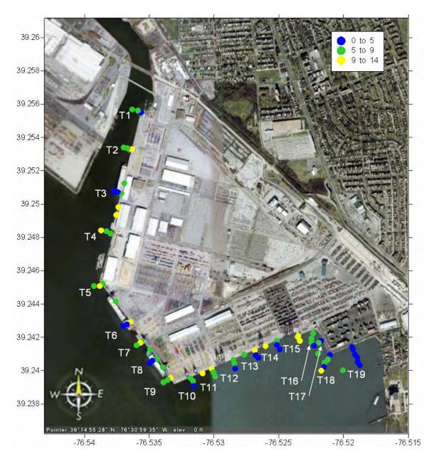
Figure 3-5. Trident subsurface conductivity distribution (mS/cm).
